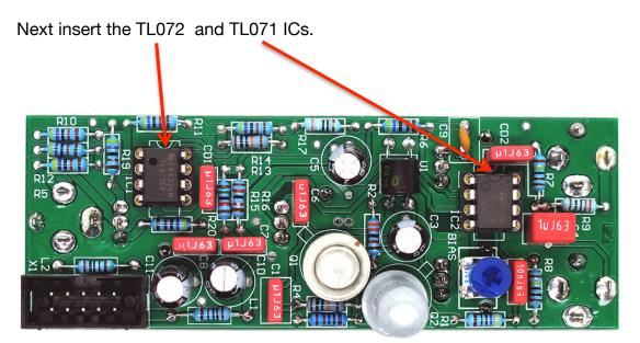
**NOTE!** – The IC orientation is vital, make sure the notch in the end of the IC or the circle mark are positioned as shown.
