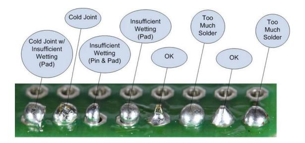
This photo is from the **Adafruit guide to excellent soldering** http://bit.ly/1jxgF3n and is reproduced under an Attribution-Sharealike
