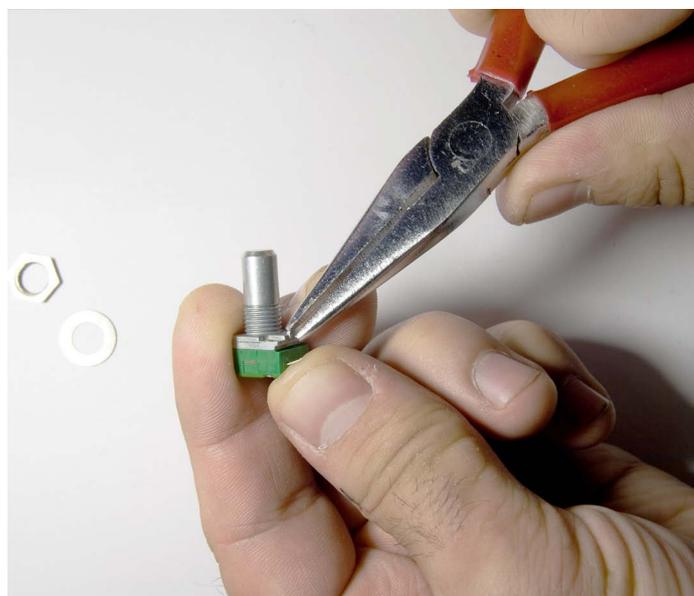
**8.** Insert two potentiometers and six jack sockets into the respective holes in the Eurorack panel. **Do not solder anything yet!** Screw on all nuts by hand. Adjust rotation of each component to direct all legs to the right (From the rear point of view)
