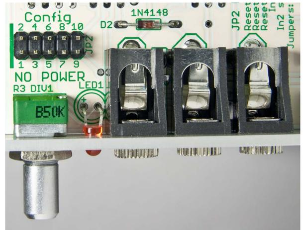
**12.** Turn each potentiometer fully counterclockwise, then install the knob. For your convenience, we have made a template, helping you to align the knob. Print the template at the original size, then cut the green shape and align it with the panel. Fit the grub screw in the knob, place the knob on the pot shaft and turn the knob according to the stripes on the template, then tighten the grub screw.
