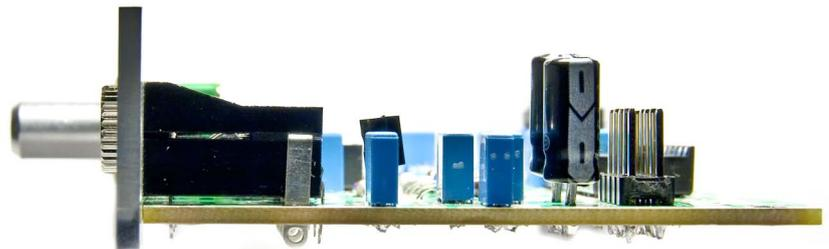
**11.** Bend the leads of the two light-emitting diodes as shown in the picture. Notice the longer lead identifying the anode. Then insert the diodes to make them fit into the hole on the front panel. Push them in if necessary. Then solder.
