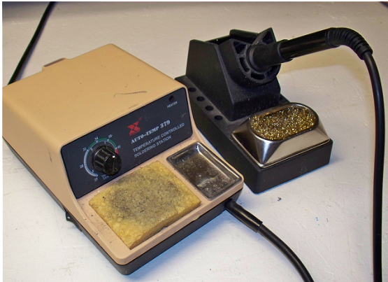
Figure 2-10. Typical temperature-controlled soldering station
