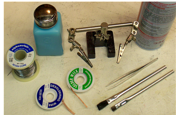
Figure 2-11. Tools you'll need for soldering
