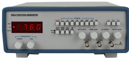
Figure 2-9. A typical function generator
