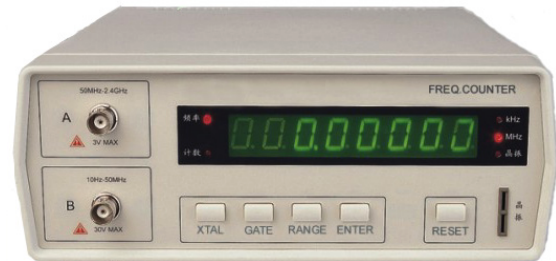
Figure 2-8. A typical frequency counter
