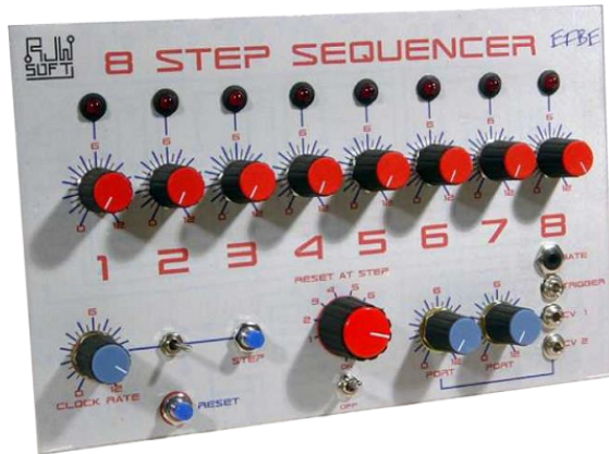
Figure 1-3. Music From Outer Space eight-step sequencer
