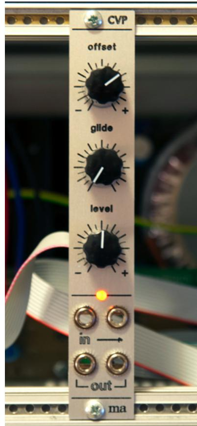
The total gain is trimmed to exactly 1.00, making the module suitable for use with pitch cvs.
