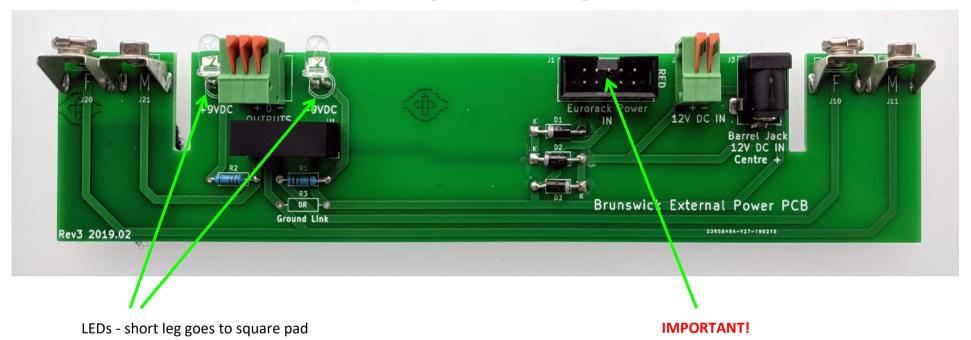
Notch on Power header must face outwards towards the edge of the PCB
