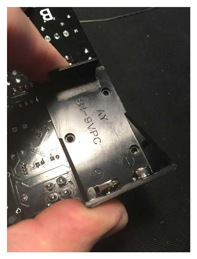
40 - Fit the battery holder to the back of the PCB - ensuring that mounting holes line up as well as possible
