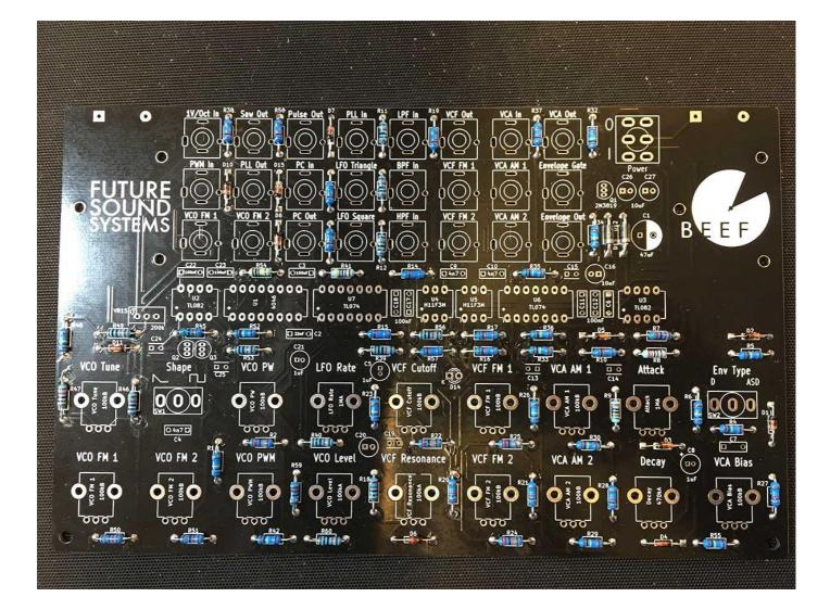
15 - Place and solder 2 x 1N4001 diodes (D12, D13)
