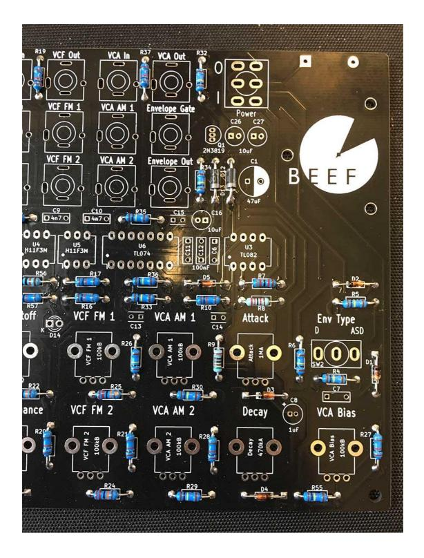
15 - Place and solder 2 x 1N4001 diodes (D12, D13) located between the 2N3819 (Q1) and rightmost TL082 (U3)
