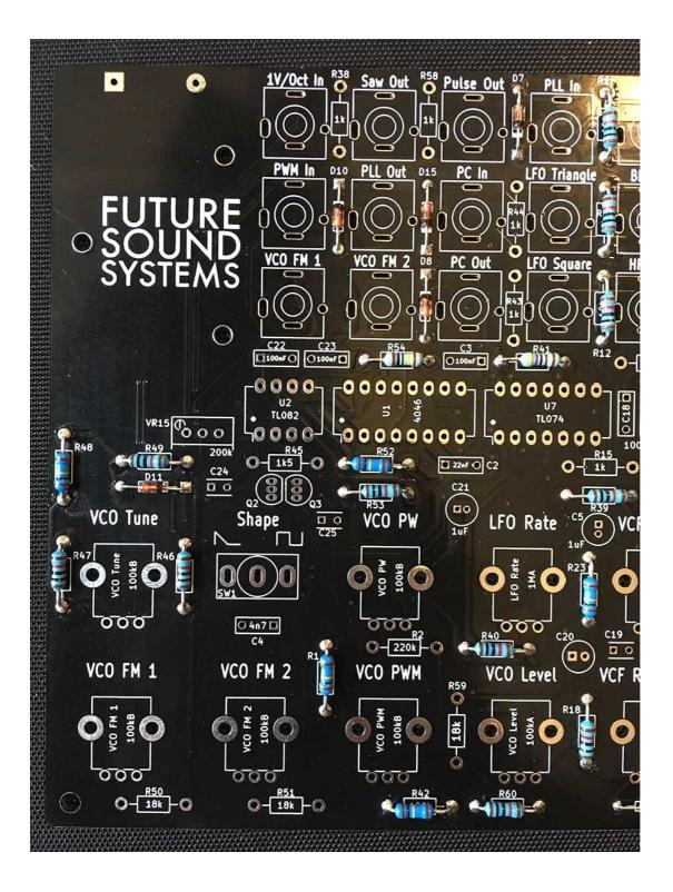
08 - Place and solder the 1M resistor at R54, located just above the 4046 (U1)
