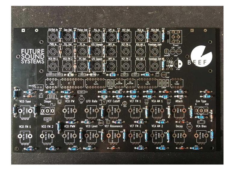
14 - Place and solder 1k resistors - these are the final resistors (R10, R14, R15, R16, R17, R19, R20, R21, R27, R28, R37, R38, R43, R44, R57)
