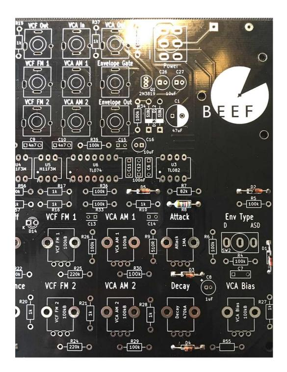
03 - Place and solder the 33k resistor at R8 – Note: IGNORE THE SILKSCREEN. THE PCB IS LABELLED 18K BUT 33K IS CORRECT
