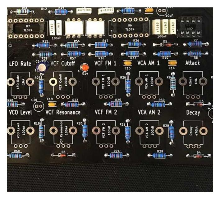
26 - Place and solder the single 2.2uF BIPOLAR cap at C5, located to the right of the LFO Rate text Note: C5 is labelled as 1uF on the PCB but 2.2uF is the correct value to use
