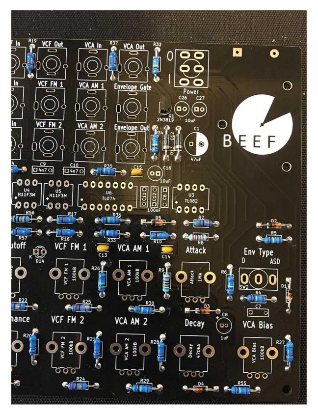
20 - Next place and solder the single 2N3819 at Q1. Note: Orientation is vital! Be sure to match the curve of the transistor body with the PCB silkscreen.
