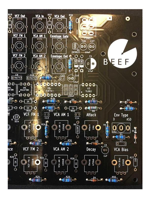
10 - Place and solder the 82k resistor at R7, located just below the rightmost TL082 (U3)
