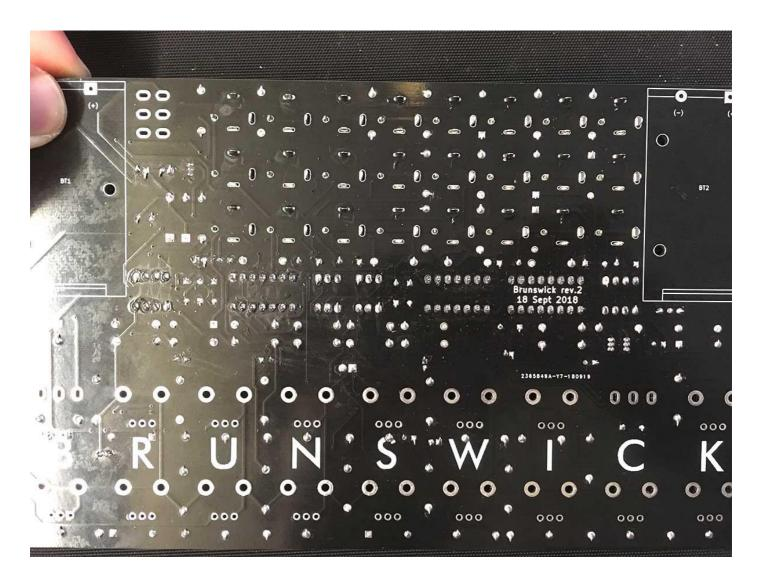
33 - Solder only the signal pin (top) lug of each jack for now – this makes them easier to desolder if there is something wrong with the build
