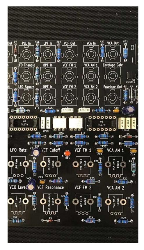
27 - Now place and solder the 2 x 10uF BIPOLAR caps at C16 and C20.jpg
