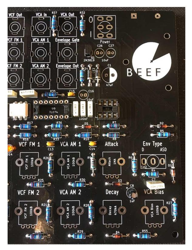
28 - Now place and solder the UNIPOLAR 1uF capacitor at C8. Note: orientation is vital for UNIPOLAR caps! The longer leg must go on the side of the + on the PCB silkscreen.
