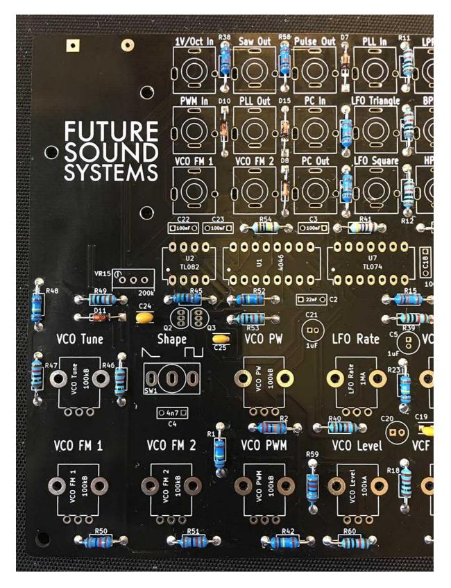
18 - Place and solder the 4.7nF CERAMIC cap at C24, located below the VR15 trimmer
