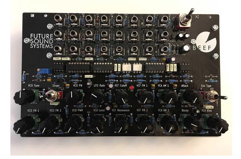
49 - Once you have tested that your build works, you can solder all the remaining legs on the jacks and pots, and then fit the knob caps
