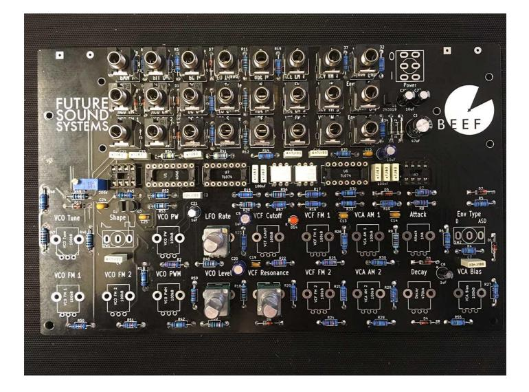
35 - Now place and solder the BOTTOM THREE LEGS of B1M pot for LFO Rate
