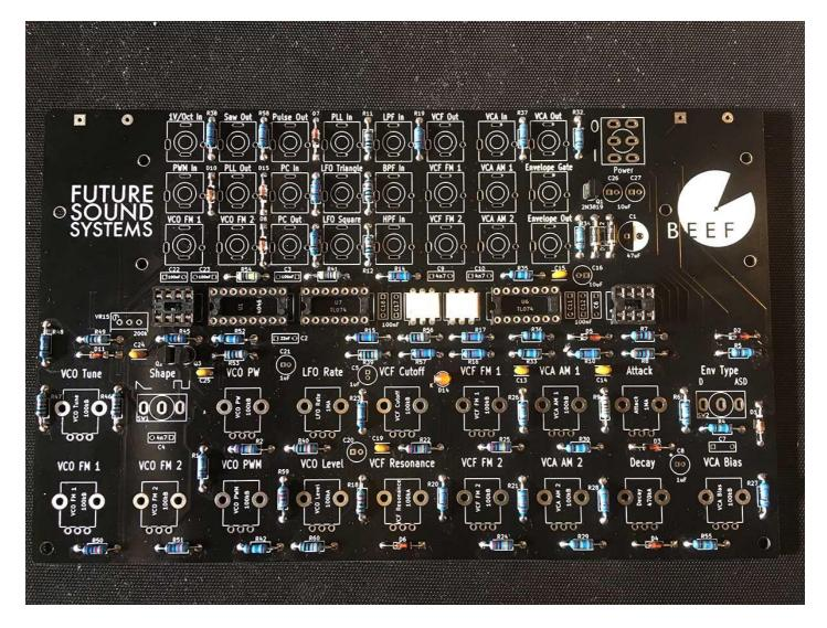
22 - Now place and solder the 3mm LED at D14. Note: Oriantation is vital! The short leg must go to the square pad labelled K
