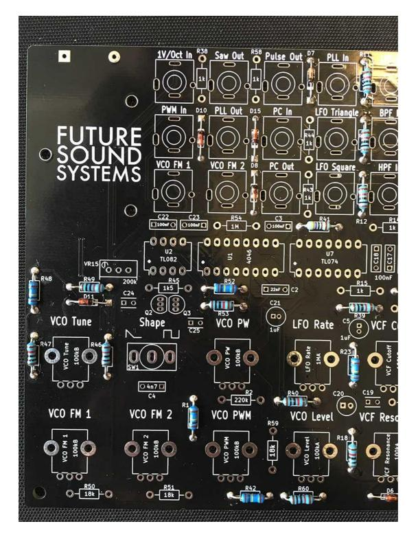
07 - Place and solder the 4k7 resistor at R41, located just above the leftmost TL074 (U7).
