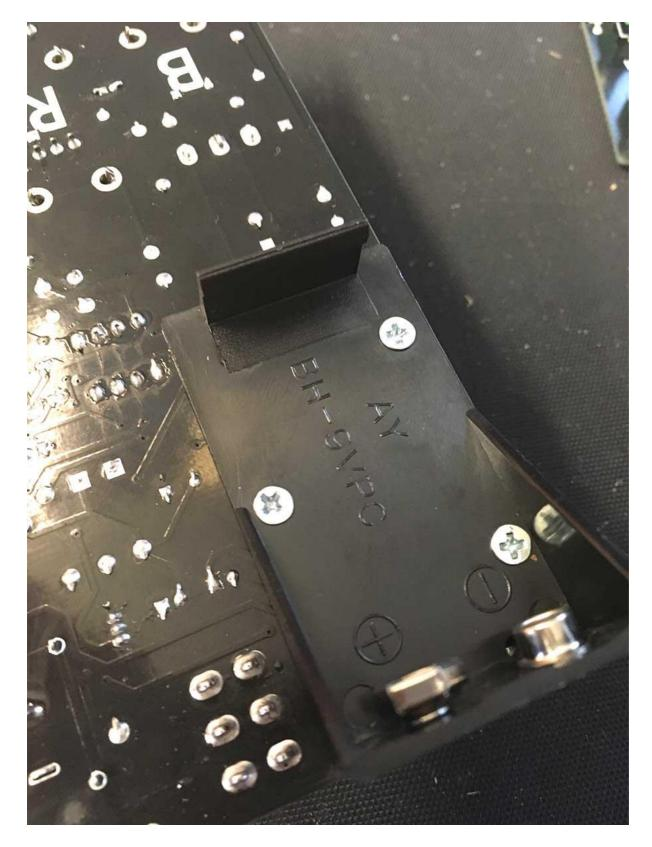
43 - Now fit the two remaining screws into each battery holder
