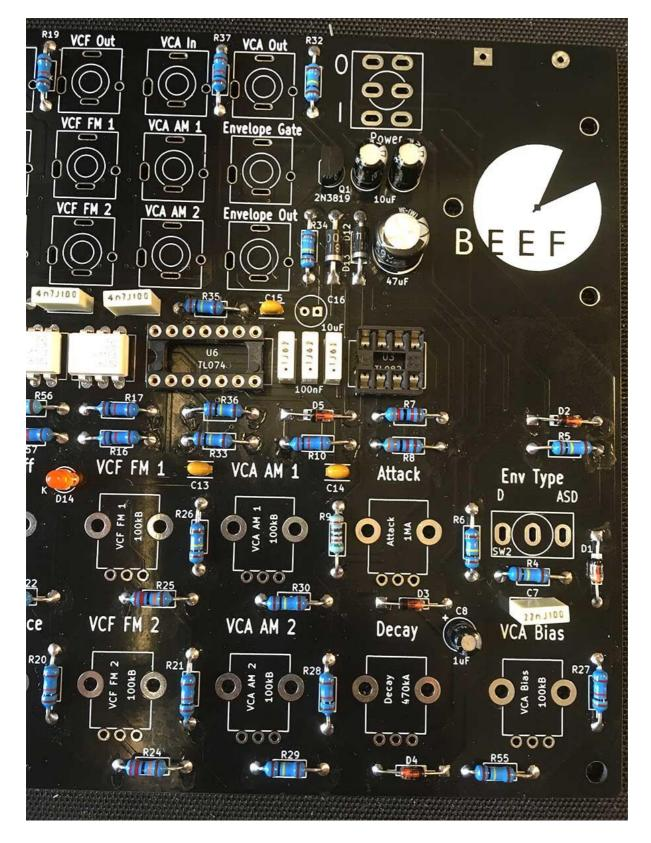
30 - Now place and solder 2 x 10uF UNIPOLAR caps at C26 and C27. Note: orientation is vital for UNIPOLAR caps! The longer leg must go to the square pad.
