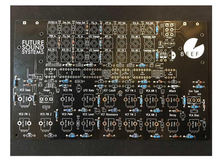
09 - Place and solder the 220k resistors (R2, R22, R24, R25)
