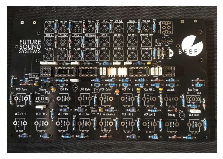
25 - Place and solder 100nF box caps at 8 the remaining box cap locations (C3, C6, C11, C12, C17, C18, C22, C23)
