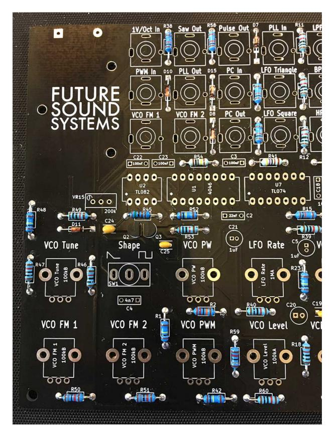
19 - Now place and solder the 2 x 2N3904 transistors at Q2 and Q3 – Note: Orientation is vital! Be sure to match the curve of the transistor body with the PCB silkscreen.
