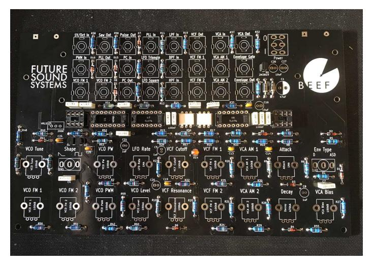
25 – Now place and solder the 100nF box caps at the 8 remaining box cap locations (C3, C6, C11, C12, C17, C18, C22, C23)
