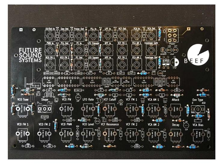
06 - Place and solder the 10k resistors (R11, R12, R13, R18, R39, R40, R46, R47, R49, R53, R56, R60)
