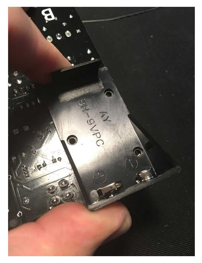
40 – Now fit the battery holder to the back of the PCB - ensuring that the mounting holes line up as well as possible
