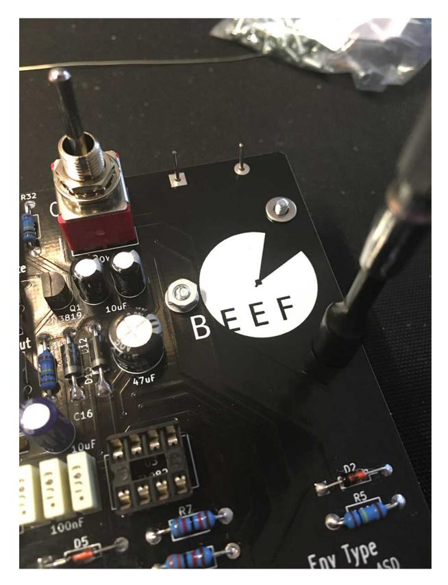
45 - Now you can fit the M2.5 nuts to each screw - a nut driver can make this easier
