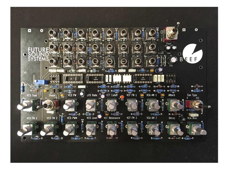
38 - Now place and solder 2 x SPDT switches and 1 x DPDT switch - ensure they sit as flat as possible against PCB
