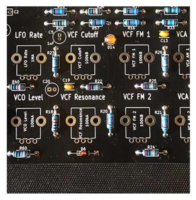
22 - Now place and solder the 3mm LED at D14. Note: Orientation is vital! The short leg must go to the square pad labelled K
