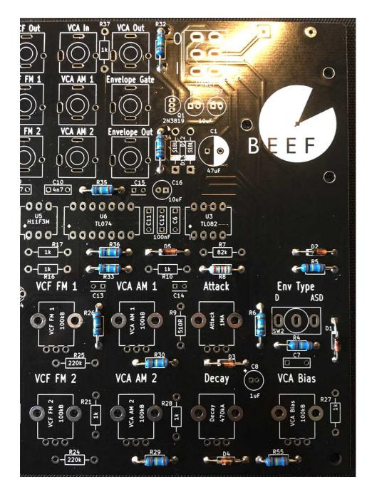
05 – Don't forget to give R55 a 100k resistor, it's located at the bottom right of the PCB
