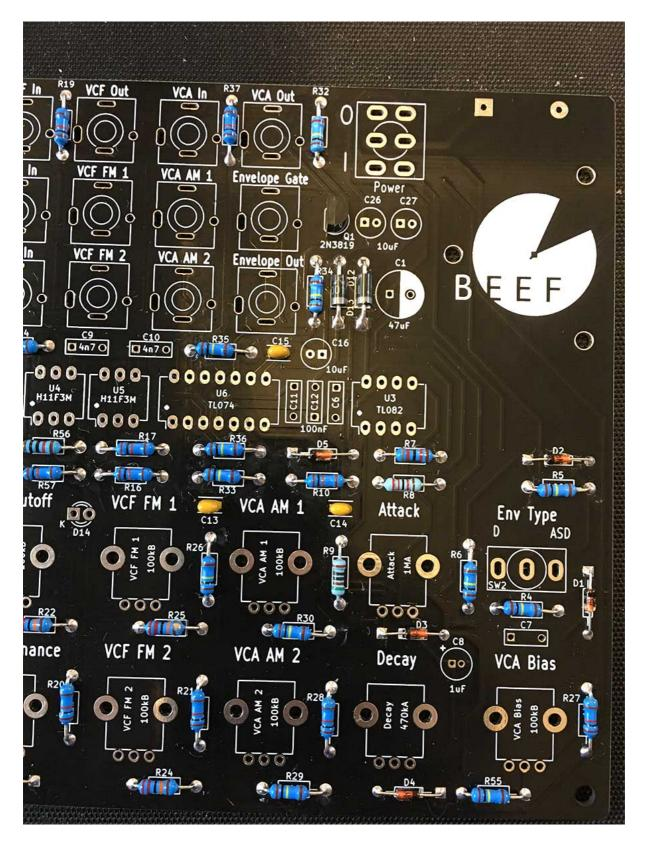
20 - Next place and solder the single 2N3819 at Q1. Note: Orientation is vital! Be sure to match the curve of the transistor body with the PCB silkscreen. The 2N3819 can be found in the silver IC bag.
