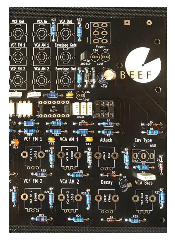
29 - Next place and solder 47uF cap at C1. Note: orientation is vital for UNIPOLAR caps! The longer leg must go to the square pad (black) the short leg to the round pad (white)
