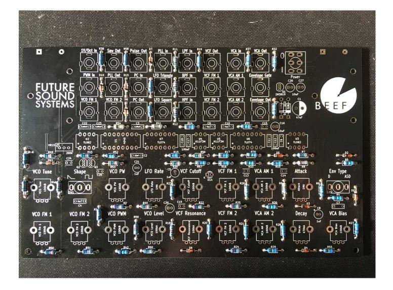
14 - Place and solder the 1k resistors - these are the final resistors (R10, R14, R15, R16, R17, R19, R20, R21, R27, R28, R37, R38, R43, R44, R57, R58)
