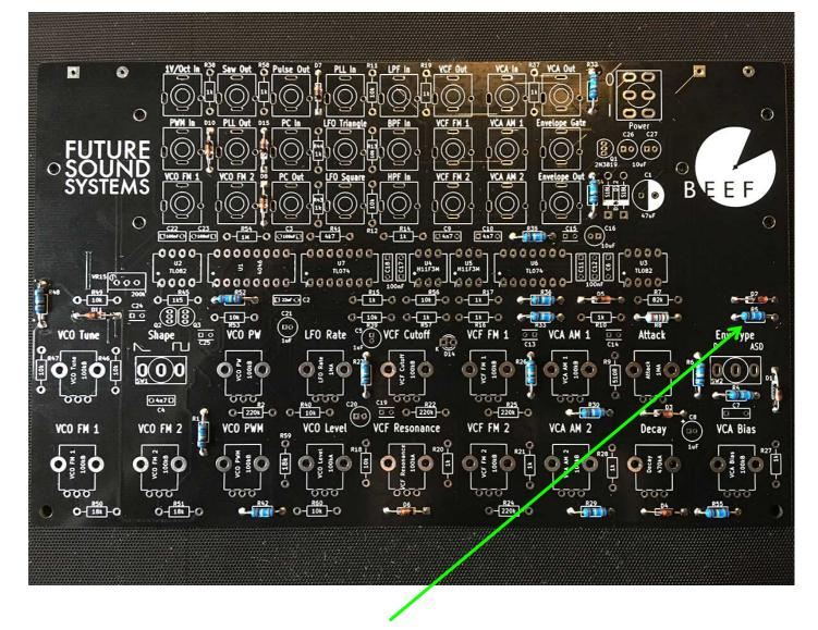
04 - Place and solder the 100k resistors (R1, R4, R5\*, R6, R23, R26, R29, R30, R32, R33, R34, R35, R36, R42, R48, R52, R55)
