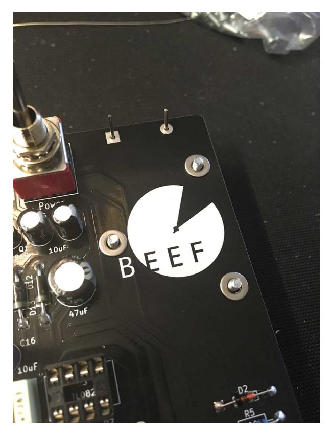
44 – Next add the M2.5 washers to each screw on the front side of the PCB. Thonk kit washers may be plastic.
