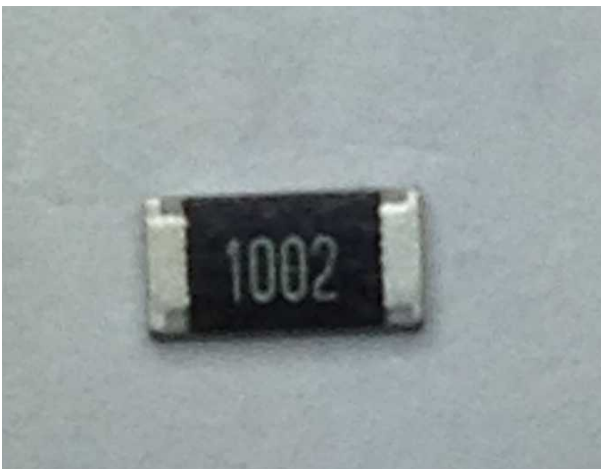
Illustration 8: 10K SMD resistor top view showing the value "1002".
