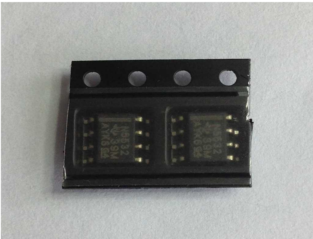
Illustration 3: SMD IC's in tape packaging
