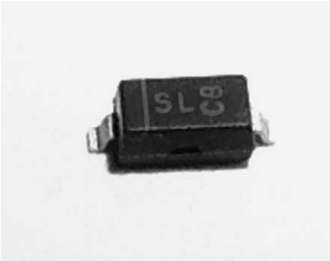
Illustration 20: Surface mount diode facing upwards, showing the angled pins, and the line identifying the cathode end (in this case on the left hand pin)
