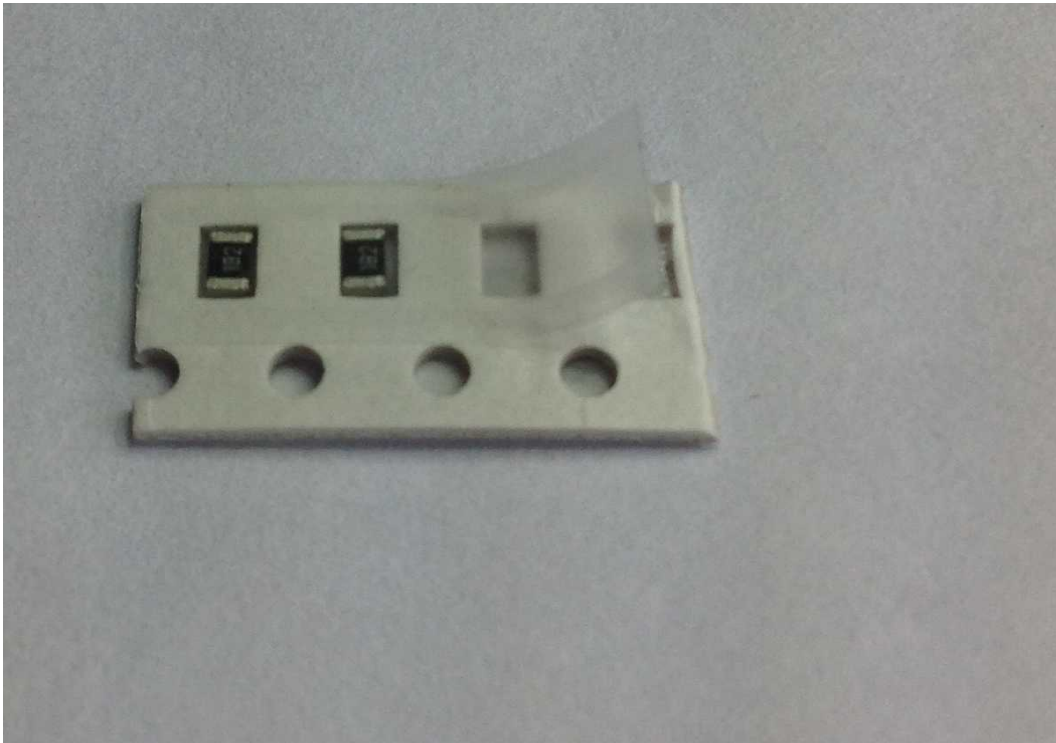
Illustration 2: SMD resistors in tape showing plastic cover partially peeled away
