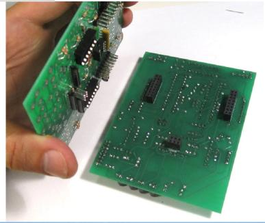
D. Gently press the boards together. Verify that everything is straight and none of the headers are at an angle, and no pins are sticking out.
