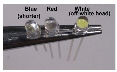
E. Look closely at the 6 LEDs. The ones with short leads are Blue, the ones with milky off-white heads are White, and the clear, long ones are Red. Insert the LEDs into the PCB where marked. The longer lead goes in the square hole.
