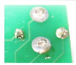
B. Once the panel is on, hold everything together with one hand while putting a nut on the four corner jacks with the other hand. This is tricky and you may drop the nut a few times: don't worry, this is the hardest part. Tighten the nuts down **slightly (1/16 turn)** with a 5/16" socket or pliers (be careful not the scratch the panel!).
