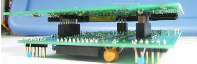
F. Now, squeezing the boards together so the female headers don't fall out, flip the boards over and solder the female headers
