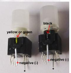
C. Look closely at the six buttons. Four are marked with a yellow mark and two are marked with black. See the photo on left. The side with the black or yellow mark is the negative side. On the PCB, this side is marked with a minus sign (-) as well as the name of the color that should go in that hole. *Note: Green and Yellow are considered the same color.* Insert the buttons into the PCB, being careful that they go in the right way and that no pins are bent.
