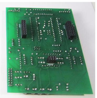
B. Flip the smaller board over so the resistors, sockets, etc are facing down. Insert the 3 female headers as shown. **Do not solder yet!**
