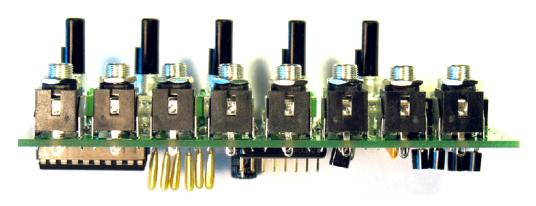
Double-check that all the pots, jacks, and LED buttons are square and flush to the PCB. The LED buttons especially will tend to fall out, so keep an eye on them.
