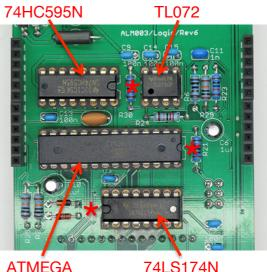
The ATMEGA chip comes preprogrammed with the SID GUTS firmware.
