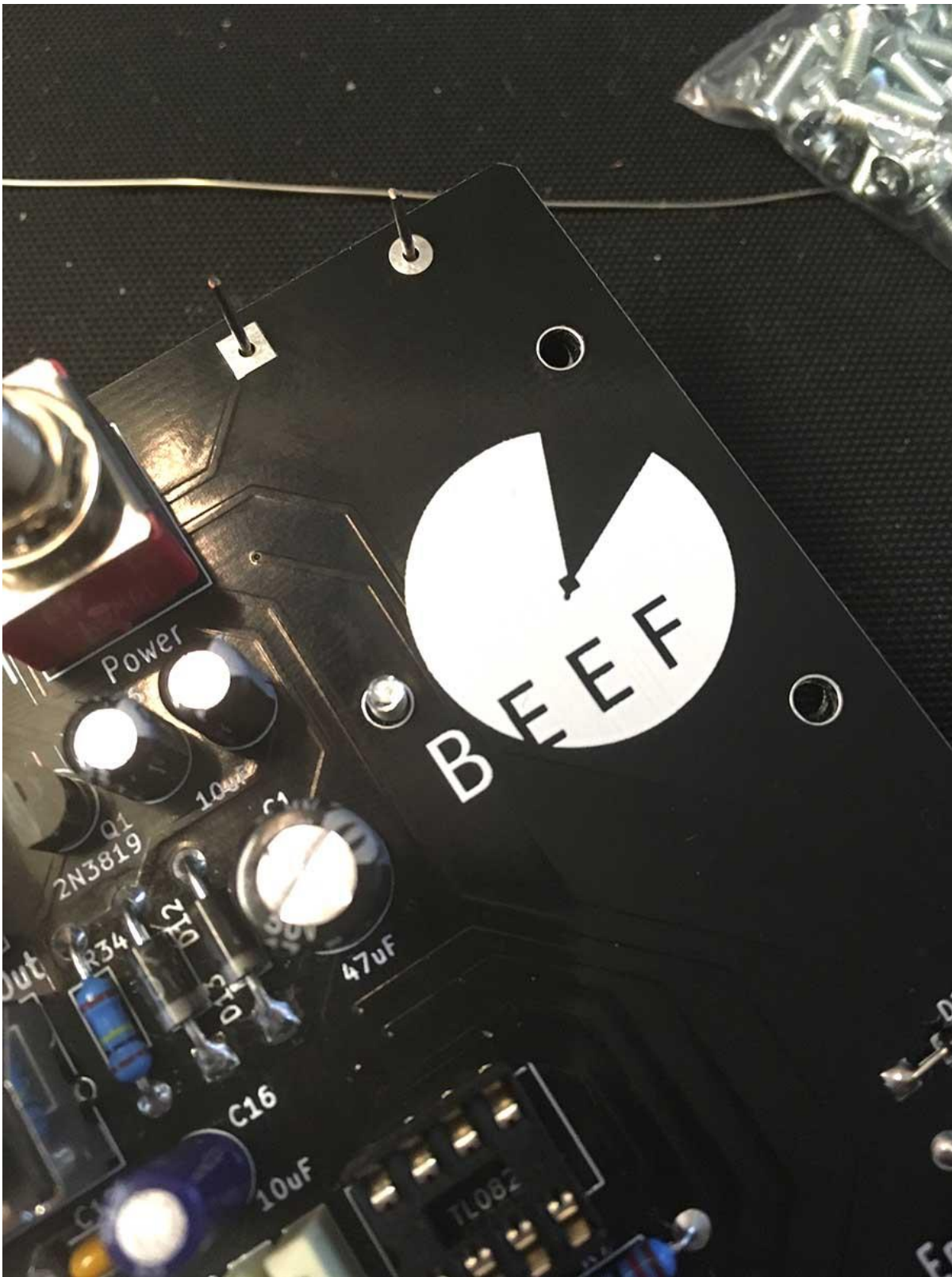
42 - The top side of the PCB should still look good once threaded
