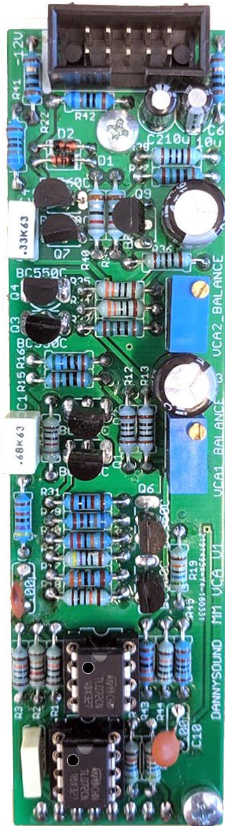
35) - 2 x TL072 opamps - orientation is vital, for these opamps match the dot with the notch on the PCB silkscreen and IC Socket
