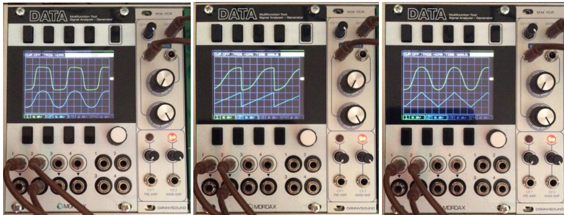
Scope plots showing soft clipping characteristics. Top trace – VCA Output, Lower trace – VCA input.
