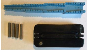
The blue bending guage is for bending the resistor and diode legs to the right size. The black IC straightener is for straightening pins of op-amps etc. The silver standoffs are 25mm Female to Female.
