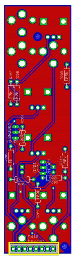
41 - MALE 1x8 pin header – this header is placed on the **same side** of the PCB as the resistors and transistors
