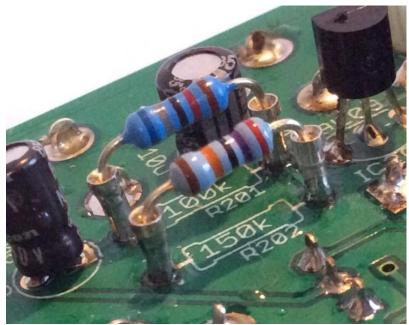
Cutting the pins from a SIL connector and soldering as shown above is useful for experimenting with different component values if you want to try out any of the modifications.
