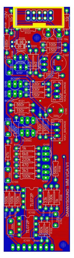
33 – 1 x SHROUDED 2x5 pin header - **make sure the slot is facing <u>away</u>** from the edge of the PCB as indicated above. Orientation is vital!
