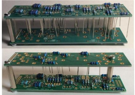
The top picture is for stuffing the Outer Board. It has the advantage of being much quicker to place all the resistors etc and it's easy to fix any mistakes. You can then solder everything from the top in one go (make sure you have decent temp. solder iron with not too fat tip!). Then unscrew the standoffs and clip all the legs. Reverse both boards as in the lower picture for the Pots Board.
