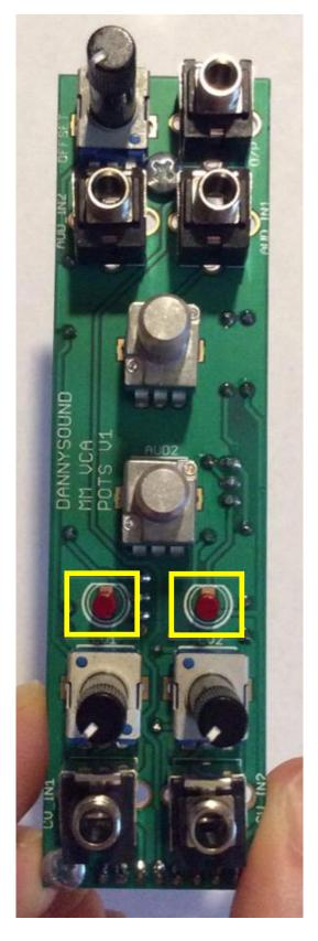
46 – 2 x 3mm Red LEDs – **NOTE:** orientation is vital, the shorter leg of the LED should go to the square pad and flat side of the PCB silkscreen diagram.
