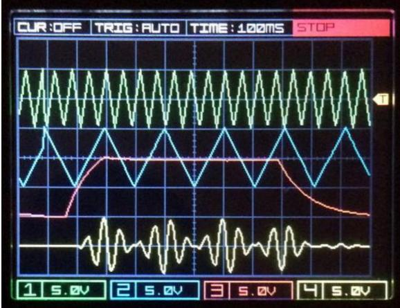
Channel 1 (Green – Top trace) – Audio input. Channel 2 (Blue – Below Top Trace) – LFO connected to CV 1. Channel 3 (Red – Below Channel 2) – Envelope connected to CV 2. Channel 4 (Yellow – Lower Trace) – VCA output.
