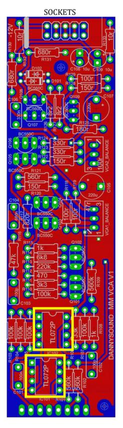
–  $2\,x\,8$  pin IC sockets - make sure the notches in the sockets match the notches on the PCB silkscreen.
