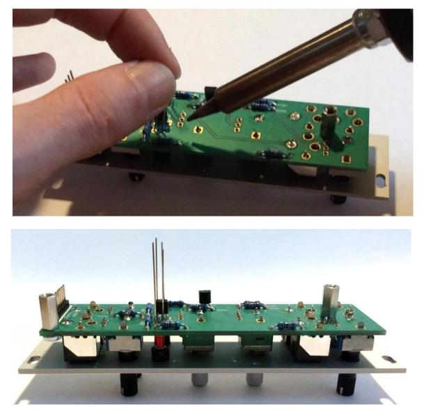
48 – Solder one leg of each of the LEDs, you can then reflow the solder to that pin while holding the LED legs to position it against the light pipe.
