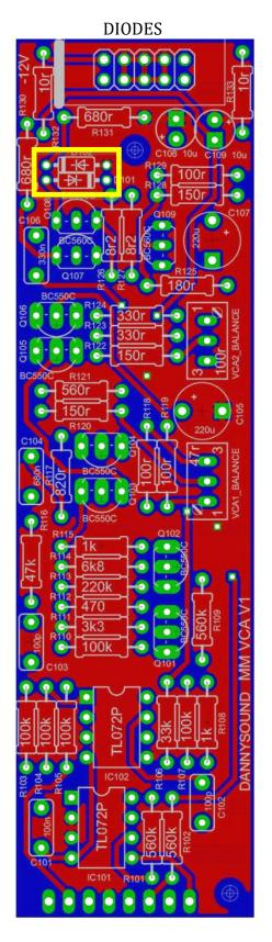
19 – 2 x 1N4148 (D101, D102) **NOTE:** orientation of this part is vital - be sure to match the line on the component with that on the PCB silkscreen
