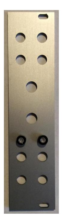
43 – Install 2 x Light pipes and retaining clips
