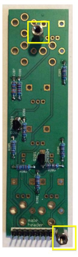
42 - 2 x Female to Female 11mm Standoffs – screw both standoffs to the PCB
