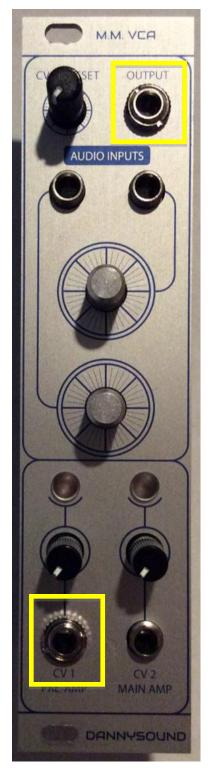
47 – Fit the panel in place, then while holding everything together turn over and solder one pin of the lower CV 1 jack socket and one pin of the output jack socket.
