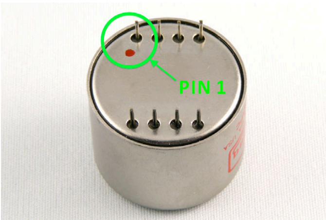
Match this transformer lead...
