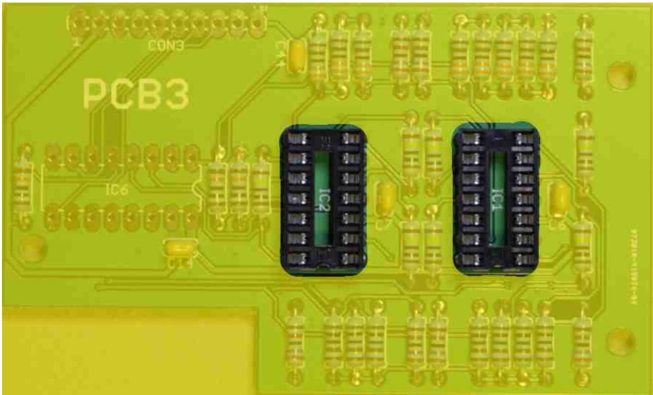
IC1, IC2 14 pin DIP sockets. IC's will be mounted later.
