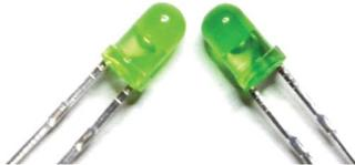
The LEDs actually need to be soldered sticking out above the board so that they protrude through the holes in the front panel. Ultimately the height is up to you, but we recommend mounting them so that they are flush with front surface of the front panel. If you mount them so that they stick out, they tend to get in the way when you are trying to push buttons.
