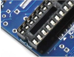
Flip the board over and solder one pin on each corner of both sockets. This makes it easy to reposition the sockets in case they aren't seated all the way down against the board; just reheat the corner pins and adjust the socket positions as necessary.
