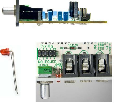
12 . Turn each potentiometer fully counterclockwise, then install the knob. For your convenience, we have made a template, helping you to align the knob. Print the template at the original size, then cut the green shape and align it with the panel. Fit the grub screw in the knob, place the knob on the pot shaft and turn the knob according to the stripes on the template, then tighten the grub screw.
