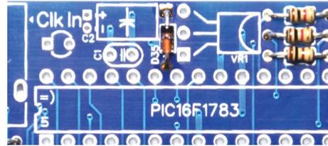
Flip the board over, solder the diode leads, then trim them just above the solder joint.
