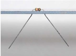
Flip the board over, solder the resistor leads, then trim them just above the solder joint.
