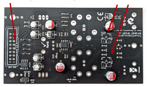
3. Next turn over the PCB and place but <u>don't solder yet</u> the 2 x LEDs. <u>Mind polarity:</u> The long leg must go to the square pad. Before soldering the LEDs place the white tube sockets - the LEDs sit in the centre of each socket. Turn The PCB over and push the LEDs through so that the LED bulb sits roughly level with the top of the hole in the tube socket as shown below, then solder the pins of both LEDs and sockets.
