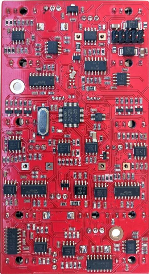
1. Insert the 2x5 pin power header onto the PCB on the same side as the SMD components and then solder in place.
