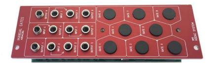
STEP 17: Tighten the jack nuts and the 2 screws.
