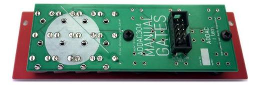
STEP 21: Finally solder the remaining pads of all jacks.
