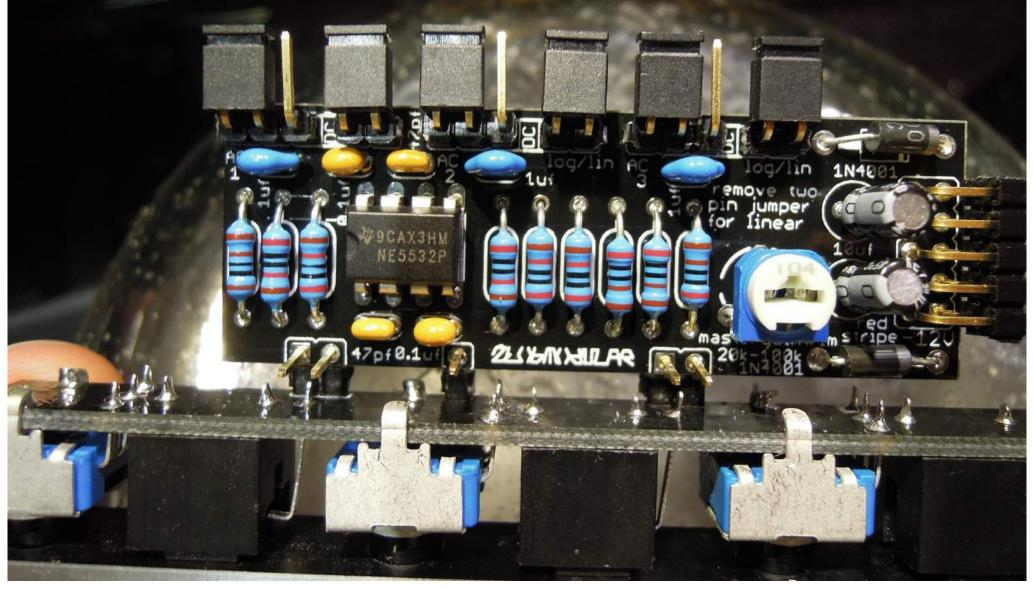
this is the configuration for DC coupling and linear operation. this configuration is better suited for control voltage mixing. the trim pot sets the master gain for all 3 channels. turn to the left for less gain or to the right for more gain. if you use a 100k trim, the center position will be around unity gain
