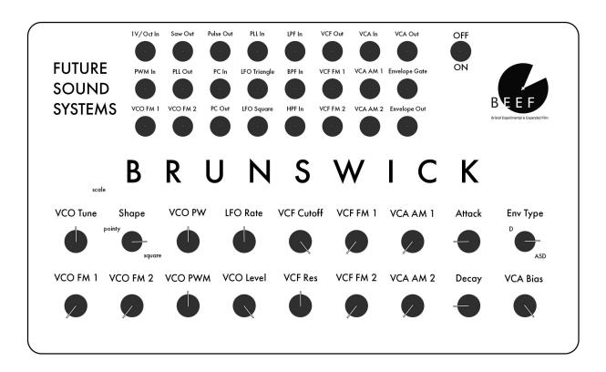
In order to check that the oscillator is working and passing through the elements of the synthesizer correctly, listen to it at each stage: "Saw Out", "Pulse Out", "VCF Out", "VCA Out". You should be able to hear the oscillator at each stage.
