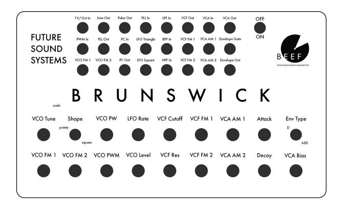
Brunswick is a monophonic subtractive synthesizer featuring one voltage controlled oscillator (VCO), one low frequency oscillator (LFO), one voltage controlled filter (VCF), one voltage controlled amplifier (VCA) and an envelope generator.
