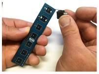
Jacks should sit flush with the PCB
