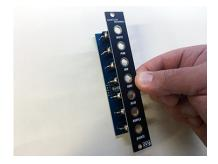
4. Solder the jacks onto the PCB.
