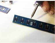
2. Insert the jacks onto the PCB
