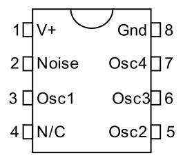
The Noise Chip saves a lot of circuitry. It is functionally equivalent to the below schematic of the Boss DR-110 noise and cymbal sound circuitry. Similar circuitry was used in all the classic analog drum machines. The DR-110, and the TR-909 used a 16-stage shift register to generate white noise. The Noise Chip uses 32-stages. The TR-808 and most other machines used a reverse biased transistor, which adds even more complexity since it takes at least 12V to get noise.
