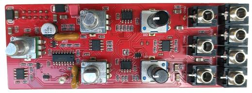
5. Now place but **DON'T SOLDER YET** the potentiometers, jack sockets and LED. **NOTE: Be sure to match the pot values with the PCB silkscreen.**
