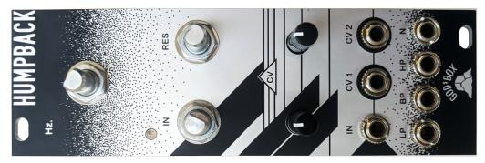
6. Now attach the frontpanel and screw on the nuts and washers to hold everything in place. Push the LED into its hole in the panel, you may want to use some masking tape to hold the LED in place while you solder. Now you can turn the module over and solder all the pots, jacks and LED. Remember - be sure that the pot values match with the PCB silkscreen before soldering!
