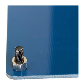
16. Next place the PCB onto the back panel inserting the four screws through their holes.
