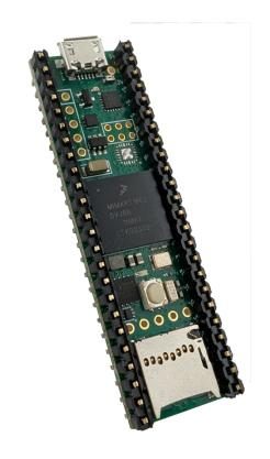
9. Now place the Teensy with the USB socket facing the edge of the PCB as shown, and gently press the Teensy pins down into the sockets until it's sitting as far down as it can go.
