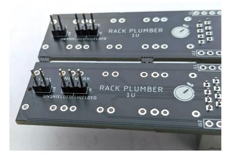
3. Then place and solder the four 1x5 male headers on the same side as the other headers, at J11 and J12. This time solder the 2 outside pins first and then check each header is flush to the PCB before soldering the rest of the pins.
