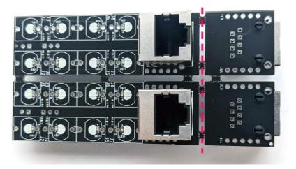
Place and solder the two 1x3 and 1x2 male headers at J9 and J10 on each long PCB.
