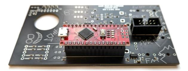
11. Next locate the LM4040 and place it on the side of the PCB without any SMD parts. Note: Orientation is vital: make sure that the curved side of the body matches the curve on the PCB silkscreen.
