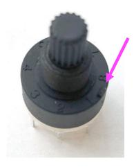
**13.** Next place but <u>do not solder yet</u> the pots and jack sockets on the PCB (remove the nuts from the jack sockets if you haven't already).
