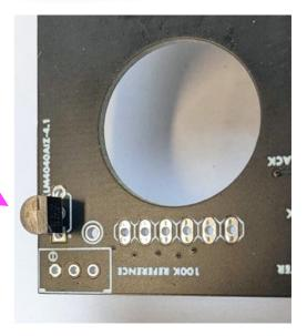
**12.** Now locate the rotary switch. It needs to have the small plastic tab cut off as shown below. Cut it as close to flush as possible. There will still be a tiny bit sticking up which is fine.
