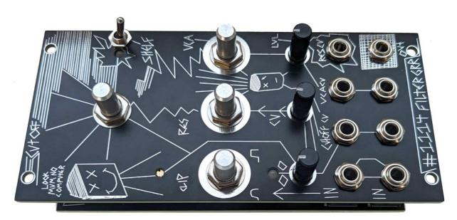
6. When all parts are soldered you can attach the knobs. Use the supplied hex key for the three small knobs and a flathead screwdriver for the large 'Cutoff' knob. Finally attach the power cable - the build is finished!
