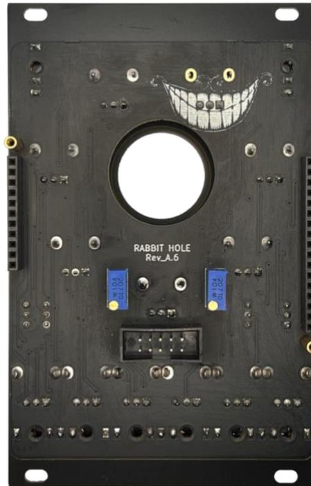
28. Give all solder joints a quick scrub with a cleaning brush to remove flux.
