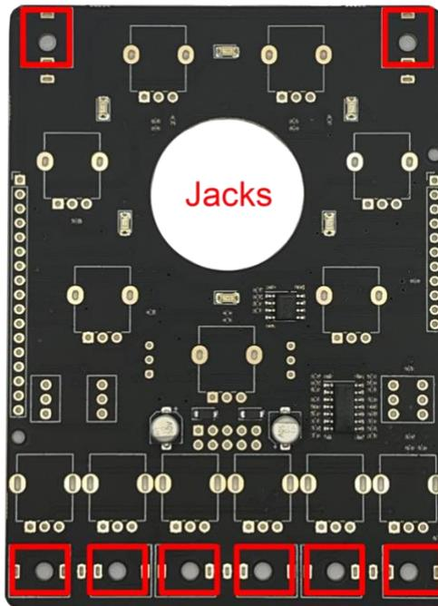
The orientation of adjacent jacks should alternate by 180°.
