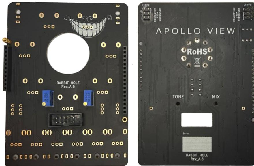
13. We will now populate the face side of the Front PCB, starting with the potentiometers for In A, In B and FB, which are all A100k (the potentiometers are clearly labelled with their value). Using pliers to straighten the kinked legs can help with positioning the potentiometers. The next four steps, 13-16, are all using the 9mm Alpha D shaft pots, which can be identified from the green body.
