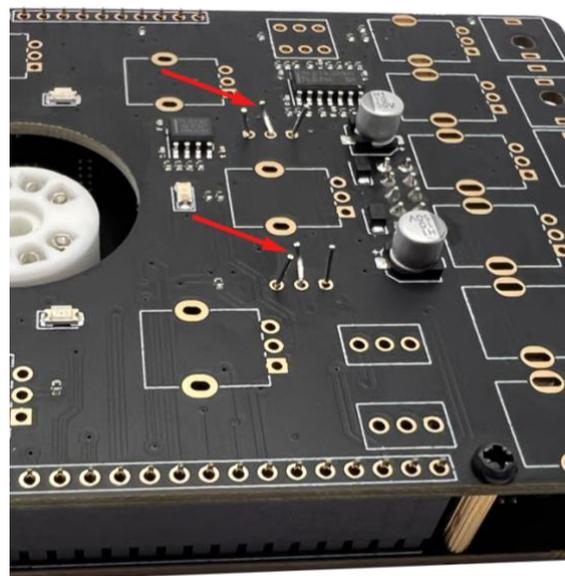
11. Solder pin headers and solder the trimmers in place.
