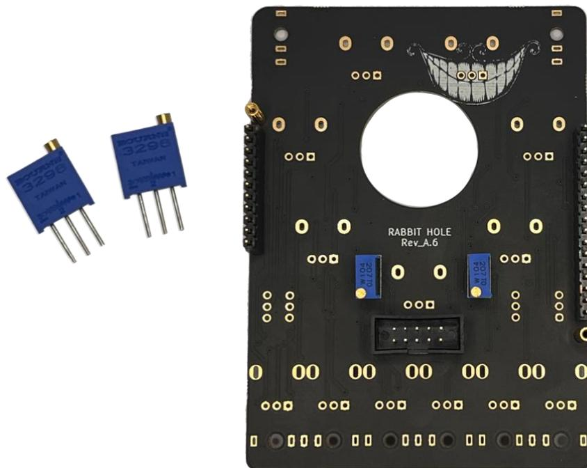
9. Lay the Back PCB face down on the pin headers. Ensure that the trimmer adjustment screws are poking through the holes on the Back PCB (give everything a wiggle until everything is correctly aligned, this can be a little fiddly, but we have confidence in your skills!). Attach Back PCB to the standoffs with the remaining two M2 screws.
