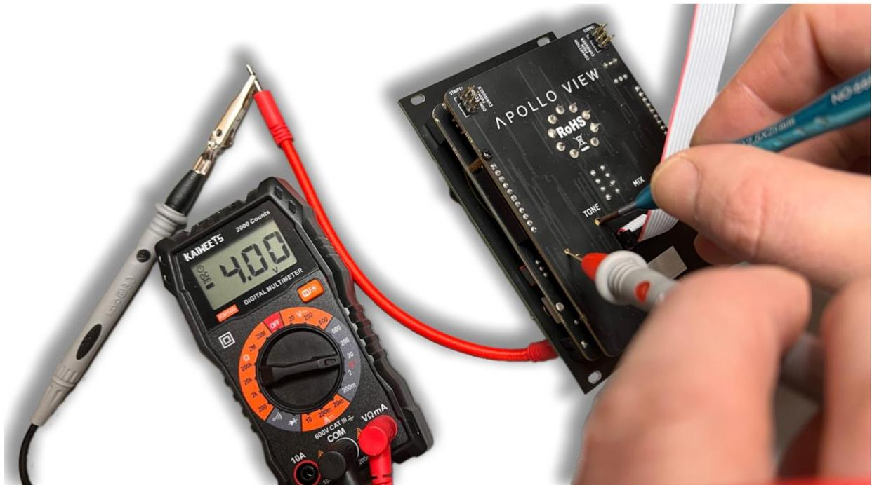
We are looking to measure -4.0V with respect to ground from each of the two test points, Mix and Tone.
