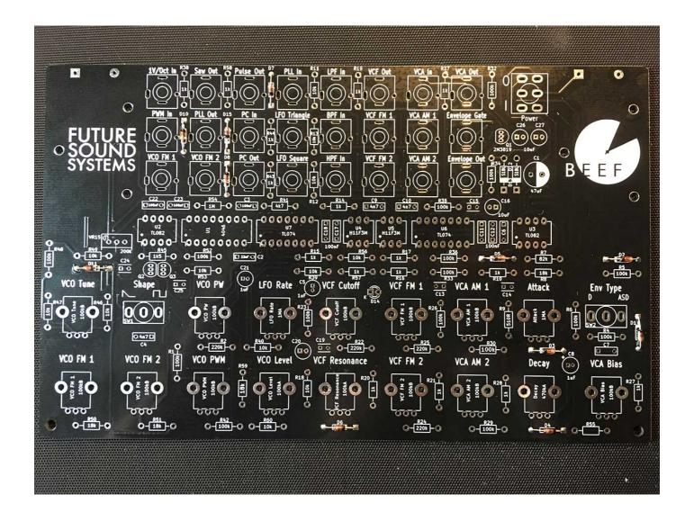
02 - First place and solder the 1N4148 diodes – Note: Orientation is vital! Be sure to match the diodes stripe with the PCB silkscreen as in the image above (D1, D2, D3, D4, D5, D6, D7, D8, D10, D11, D15)
