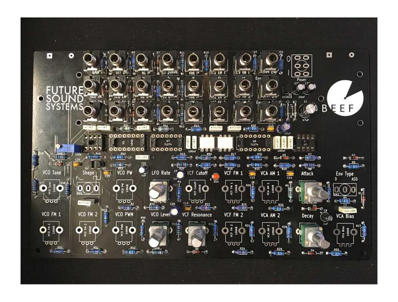
36 – Now place and solder the BOTTOM THREE LEGS of the A1M pots for Attack and Decay
