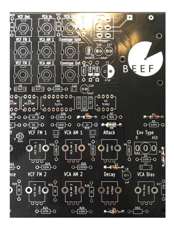
03 - Place and solder the 33k resistor at R8
