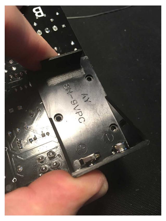
40 - Now fit the battery holder to the back of the PCB - ensuring that the mounting holes line up as well as possible
