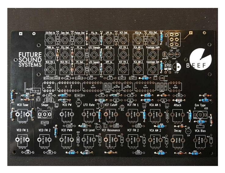
06 - Place and solder the 10k resistors (R11, R12, R13, R18, R39, R40, R46, R47, R49, R53, R56, R60)
