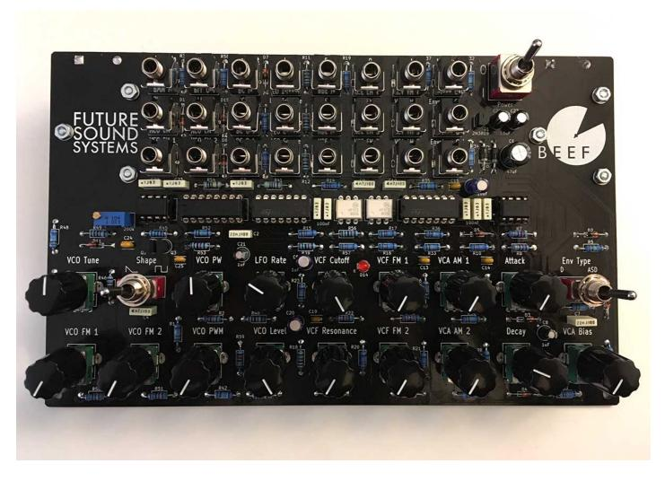
49 - Once you have tested that your build works, you can solder all the remaining legs on the jacks and pots, and then fit the knob caps
