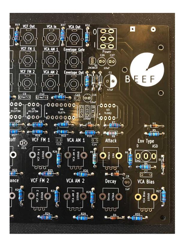
15 - Place and solder 2 x 1N4001 diodes (D12, D13) located above the rightmost TL082 (U3)
