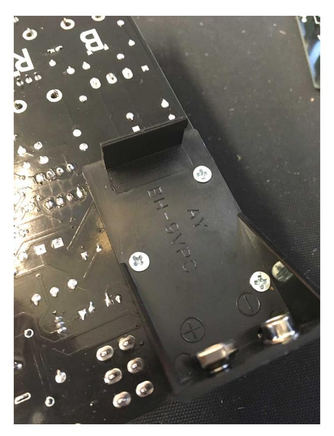
$\ensuremath{\mathsf{43}}$  - Now fit the two remaining screws into each battery holder
