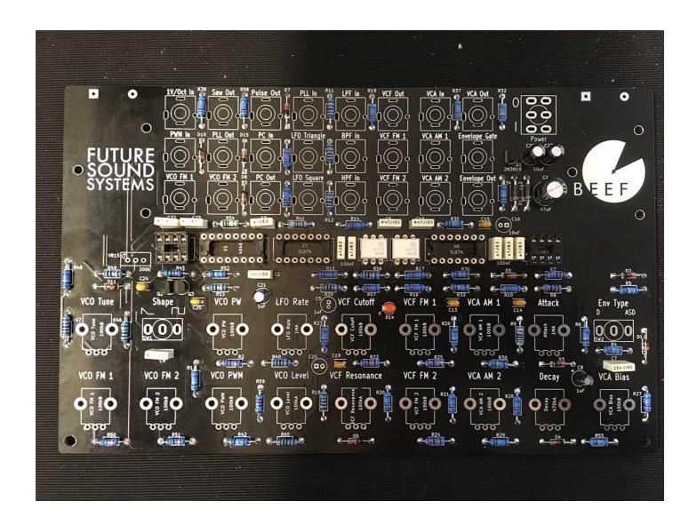
31 - Now place and solder the UNIPOLAR 2.2uF cap at C21. Note: orientation is vital for UNIPOLAR caps! The longer leg must go to the square pad.
