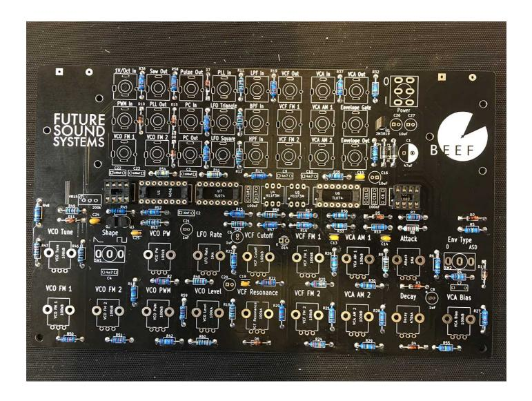
21 - Now place and solder the IC sockets. Note: Thonk kit includes 6 pin IC sockets for U4 and U5, solder these in as well. Be sure to match the notch on each socket with the dot on the PCB silkscreen.
