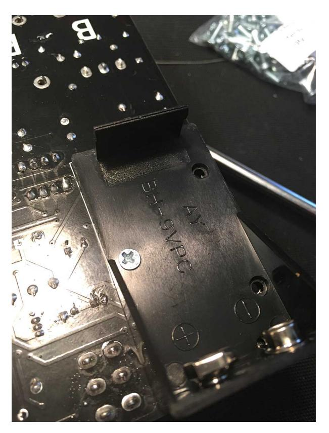
41 - Now fit an M2.5 screw to one hole to secure - you may have to thread through the PCB pad
