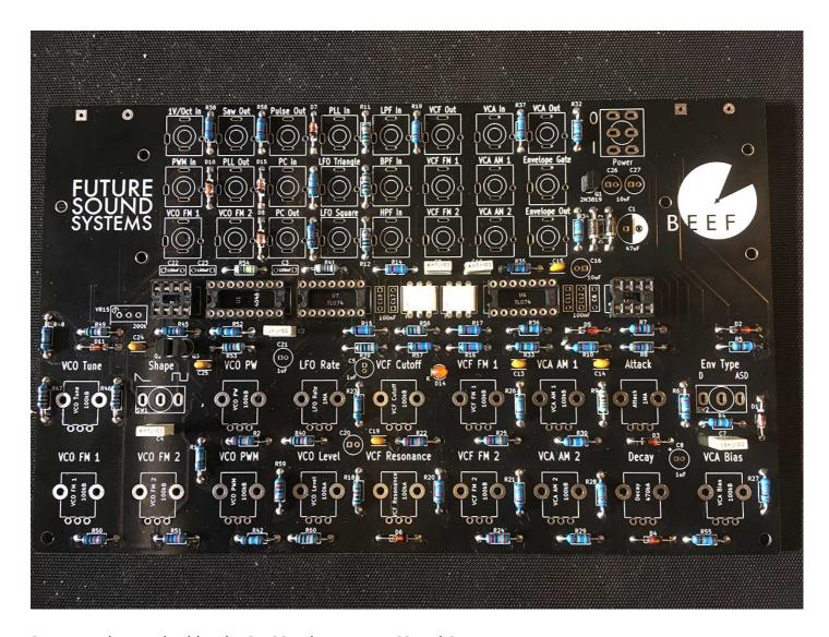
24 - Next place and solder the 2 x 22nF box caps at C2 and C7
