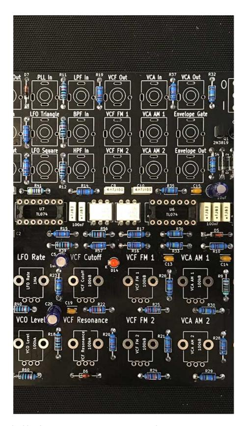
27 - Now place and solder the 2 x 10uF BIPOLAR caps at C16 and C20
