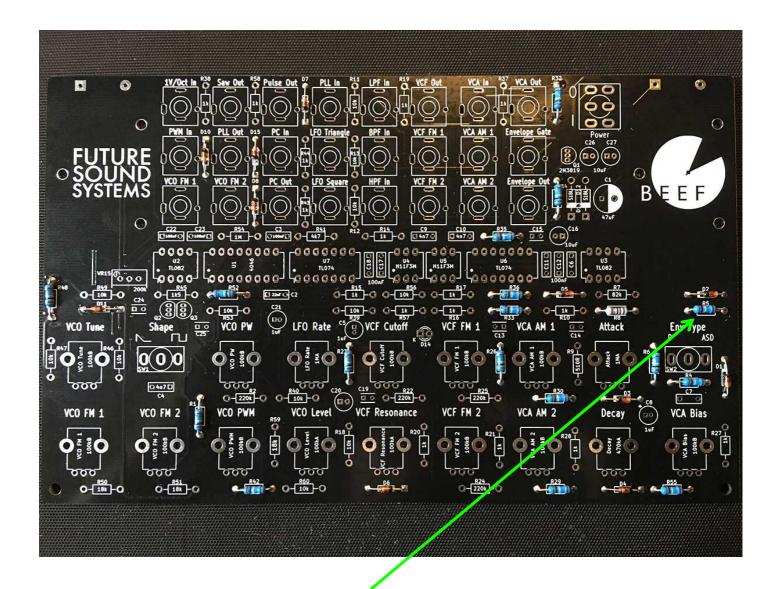
04 - Place and solder the 100k resistors (R1, R4, R5\*, R6, R23, R26, R29, R30, R32, R33, R34, R35, R36, R42, R48, R52, R55)
