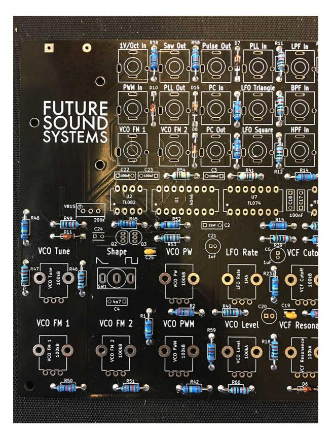
17 - Place and solder 2 x 100pF caps at C19 and C25
