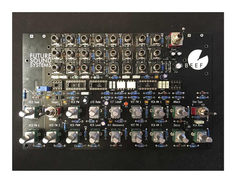
38 - Now place and solder 2 x SPDT switches and 1 x DPDT switch - ensure they sit as flat as possible against PCB
