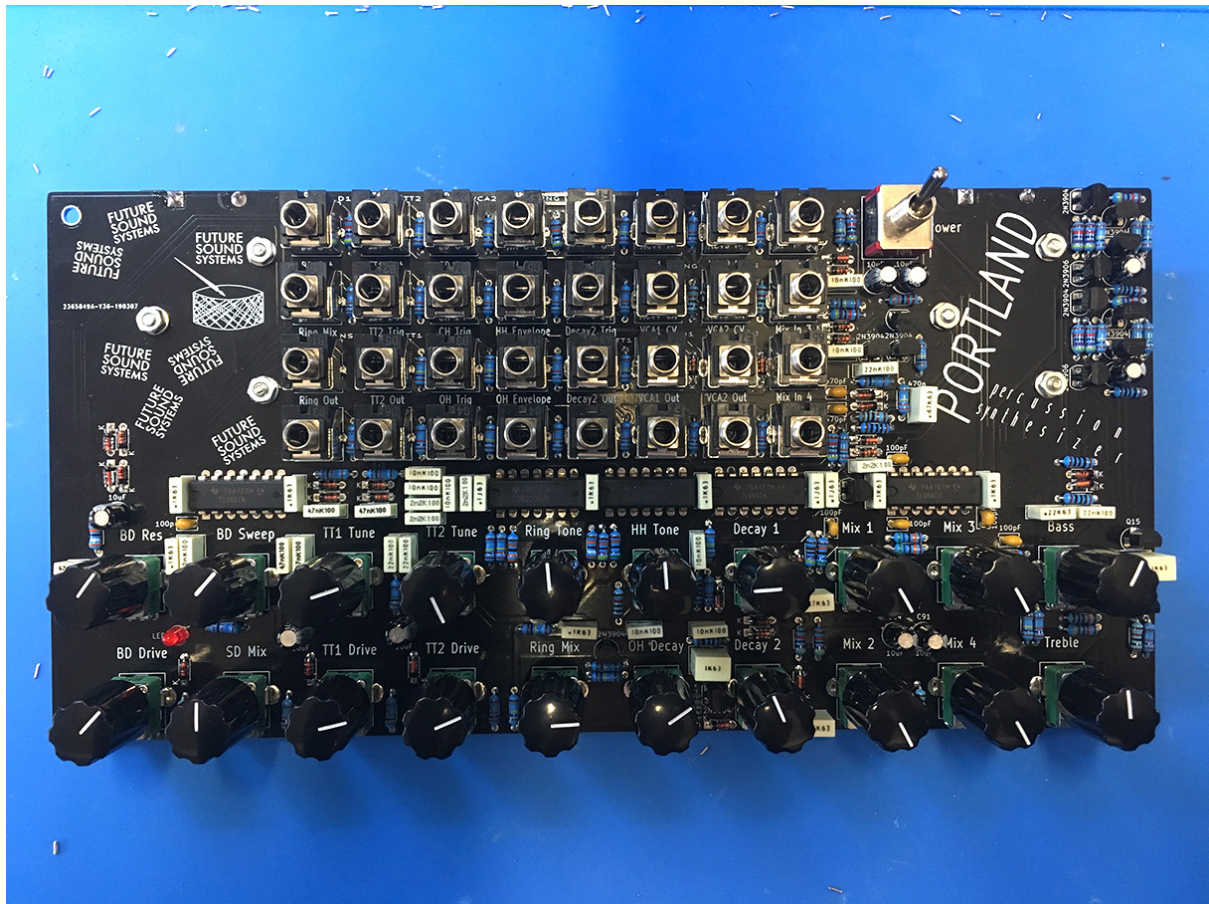
53 - Finally place the twenty knobs – the build is now finished!
