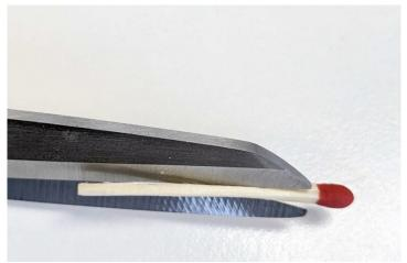
3. Insert the two halves of matchstick into the void.
