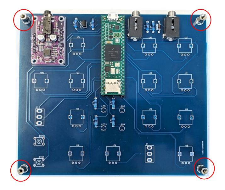
With the spacers in position locate the following parts and place <u>but don't solder yet</u> on the PCB.
