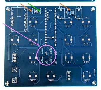
2. Locate the single 1N4148 diode and solder into the position shown.
