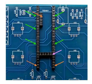
Now locate the low-profile male headers. The kit includes three lengths of 20 pins and one pre-cut length of 5 pins.
