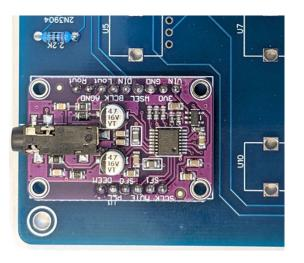
12. With the DAC Board secured to the headers you can now solder the pins on the reverse of the PCB.
