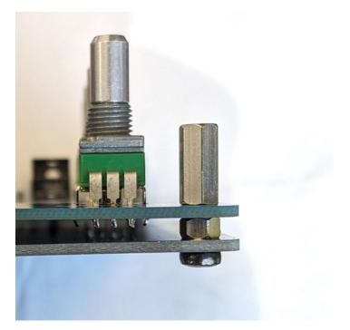
22. For the final step replace the front panel lining up all components and securing in place with the 4 x remaining 6mm black screws. Secure all pots and switches with their nuts and washers, and finally add the knobs and yellow switch caps. The build is now complete!
