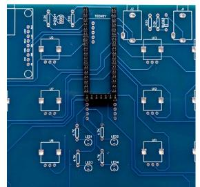
6. Place the remaining three 5 pin female headers into position.
