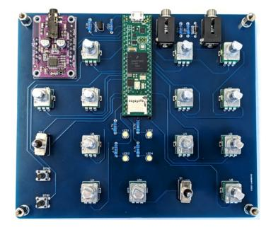
The LED's must be placed with the negative short '-' leg going to the flat side of the diagram on the PCB. The positive '+' leg of the LED should be noticeably longer.
