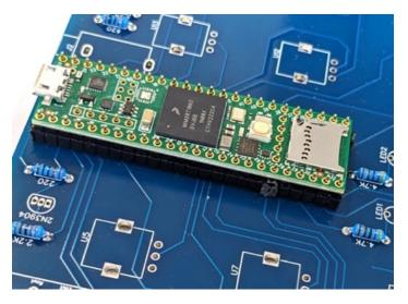
With the above steps complete flip the board over and solder two opposite corner pins of the female sockets.
