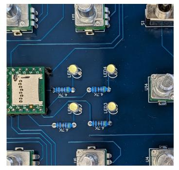
17. Place the frontpanel over the top of the components ensuring all parts are inserted fully through the holes.
