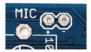
The red wire should go to the plus symbol, but if the wires get mixed up then the module will still work fine, so don't worry too much about it.
