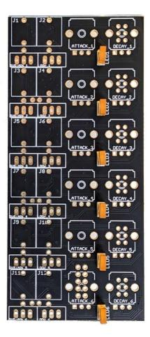
Next locate the pin sockets in the small bag. These are placed on the front PCB on the same side as the SMD pre-soldered components. **Don't solder them yet!**
