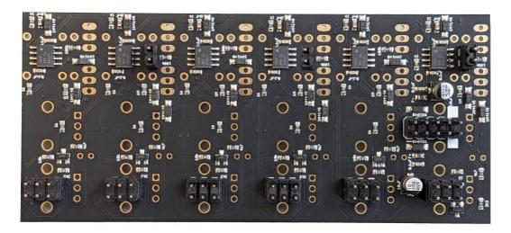
Next place the back PCB onto the pin headers to sandwich the PCBs together. You might need to wiggle the PCB slightly to ease the headers through their holes. Using pliers or a screwdriver can also be helpful to gently nudge the 2 pin headers to line up properly.
