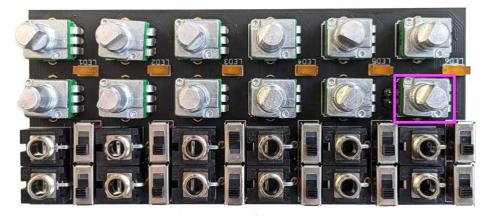
Now place the frontpanel over the components, and then secure it in place by screwing all nuts onto the jacks and black nuts onto the pots.
