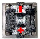
On the bottom side of each button there is a small + and - symbol that must match up with the corresponding symbols on the PCB as shown.
