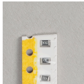
Markings on a SMD resistor
