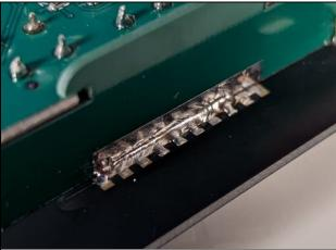
Now on to the remaining pads on the spacer PCB. The best way to solder them is to place the end of your solder wire across the pad as shown, and slowly move your (ideally very hot) soldering iron over it. However you do it, make sure there is a good connection between the panel pads and the spacer PCB pads, as this spacer will ensure the PCB does not get bent when the buttons are pressed.
