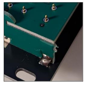
Put the spacer PCB into its place as shown. Make sure it sits perpendicular to the front panel. The solder pads on the spacer should be on the outside! It might be slightly bent, this is normal as the material is not very thick. Solder one of the corner pads first. Use plenty of heat to make a good connection. Then solder the opposite corner, bending the spacer if needed. It should now sit well in the notches on the PCB. Don't solder the remaining pads just yet.
