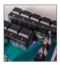
The short leg goes on the "-" side. This side is also marked with a stripe on the capacitor body.
