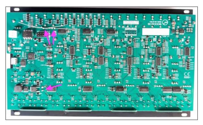
Snip off the LED and capacitor legs with a wire cutter.
