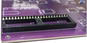
Next locate the purple DAC PCB inside its own bag. This is provided with two strips of 8 pin headers that must be split and combined to make a row of 6 and a row of 9.
