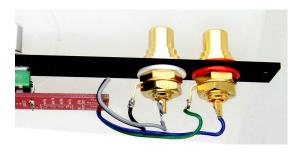
Here we show the **SEND RCA** soldered, the **black wire** on the ground ring is going to the PCB input marked **Ring**, the **grey wire** on the tip of the jack is going to the PCB input marked **Tip**.
