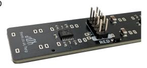
2. Check that this is soldered flush to the board by first soldering one joint and reflowing and adjusting where necessary.
