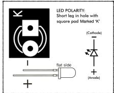
Make sure all polarised components (Diodes, LEDs, electrolytic capacitors) are placed the correct way round.
