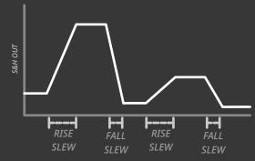
As the CV i input is used for the incoming signal, the CV ii input will control BOTH rise and fall slew rates. This CV value is summed with the SLEW UP (i) knob and SLEW DOWN (ii) knob simultaneously.
