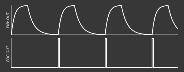
If an envelope is re-triggered while it is decaying (either in TRIG or GATE mode), the EOC will output immediately.
