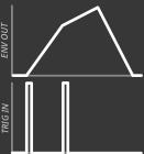
If a trigger or gate is received during the decay stage, the envelope begins a new rise from its current level. The attack time remains the same regardless of the point it restarts from.
