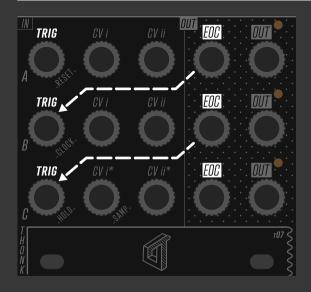
TRIPLE MOD includes normalisation between channels - each channel's EOC output is normalled to the next channel's trigger input - as indicated by the dashed lines on the panel.
