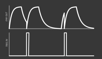
**HOLD MODE** - The LFO will only run when a HIGH gate signal is sent to the TRIG input, and will be stopped or 'gated' when the gate is LOW. The LFO will always complete it's full cycle, even if the gate goes LOW before it is finished.
