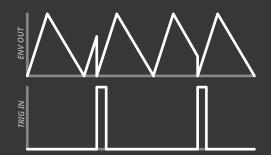
**Gate mode** - If a gate goes HIGH at any point of the cycle, the envelope will reset back to zero immediately. If a gate goes LOW at any point, the decay portion will start from the current level. If a gate is HELD high, once the envelope reaches it's max level, it is held at that level until a gate goes low again.
