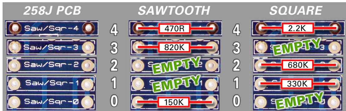
You may want to start your board by hardwiring to one waveshape first as you cannot test the board otherwise.
