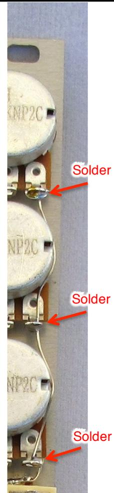
16 – Let's move onto the hookup wire. This is what you will use to make the connections between the pots and jacks.
