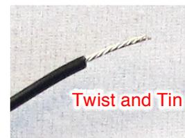
**TIP** - If you move on from this kit to more complex projects where you wire from a PCB to a front panel then I advise using stranded wire as it is more strain resistant. For jobs like the AT-AT-AT where everything is panel mounted, solid core is fine and slightly quicker to work with.
