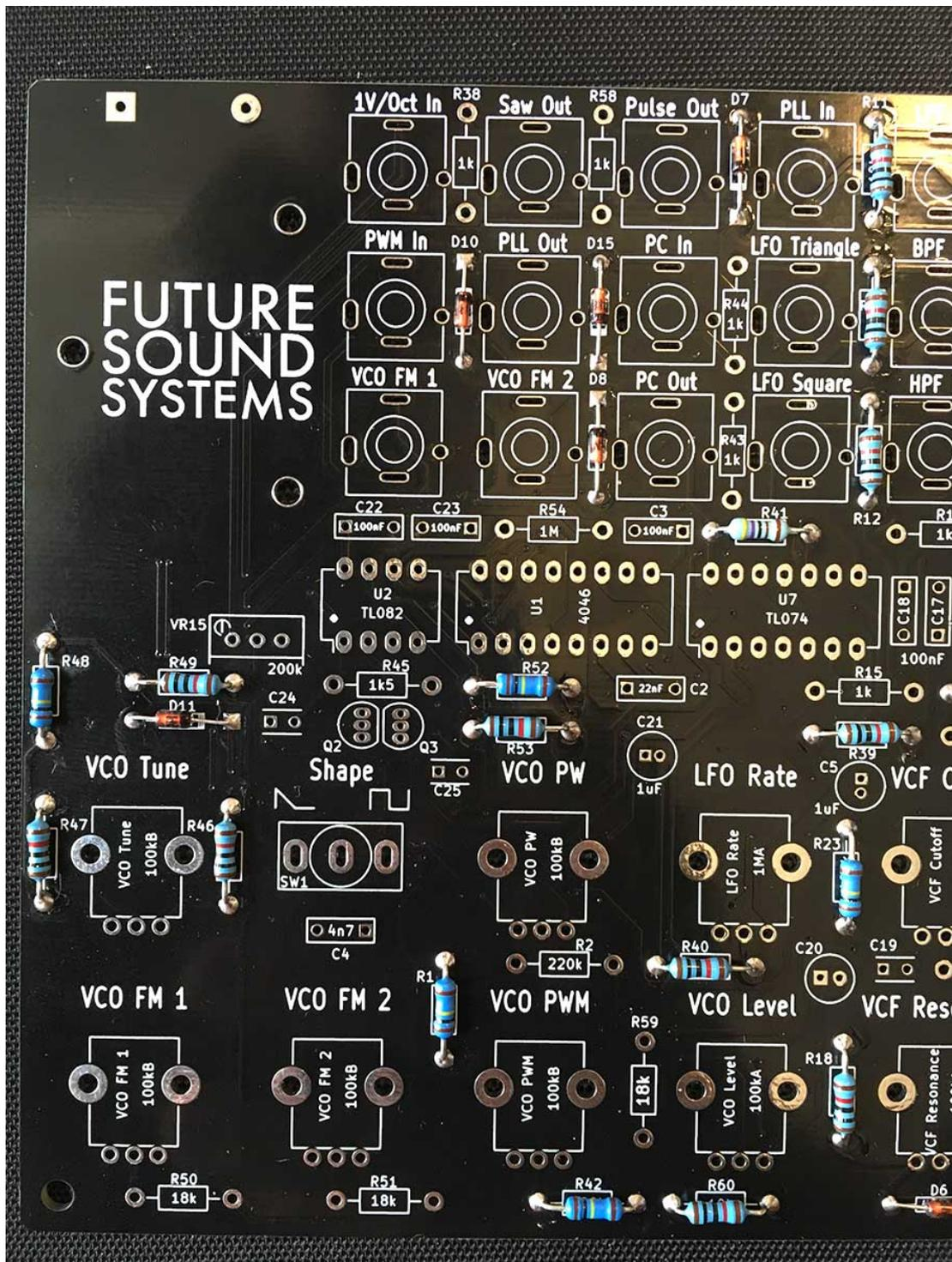
07 - Place and solder the 4k7 resistor at R41, located just above the leftmost TL074 (U7)
