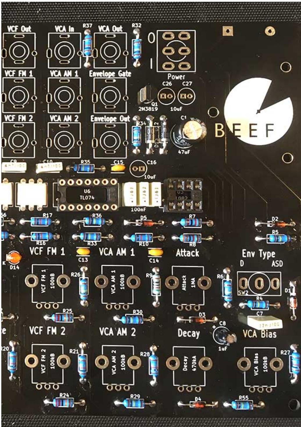
29 - Next place and solder 47uF cap at C1. Note: orientation is vital for UNIPOLAR caps! The longer leg must go to the square pad (black) the short leg to the round pad (white)
