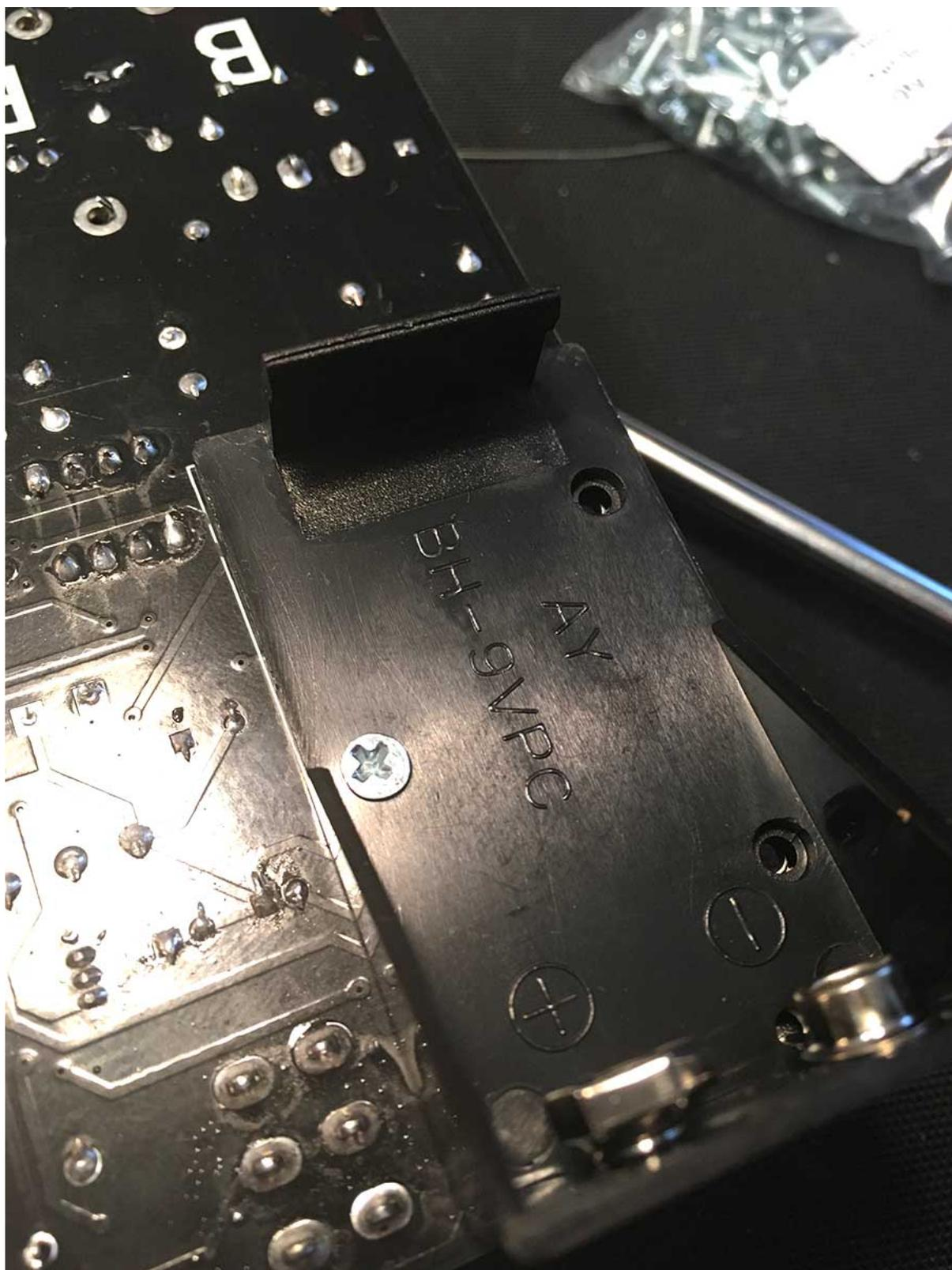
41 - Now fit an M2.5 screw to one hole to secure - you may have to thread through the PCB pad
