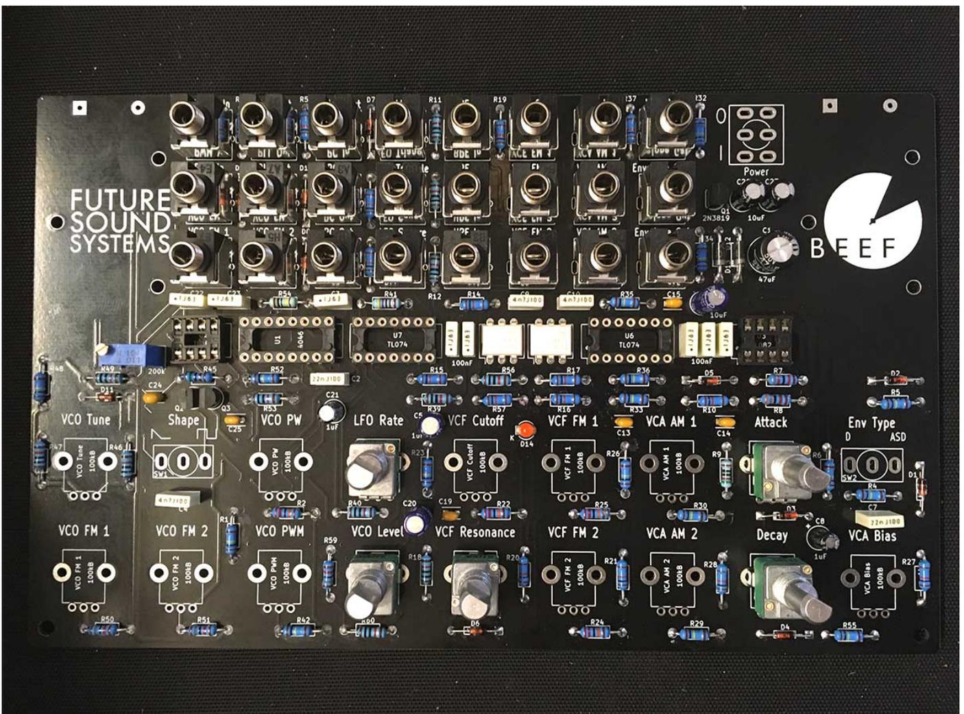
36 – Now place and solder the BOTTOM THREE LEGS of the A1M pots for Attack and Decay
