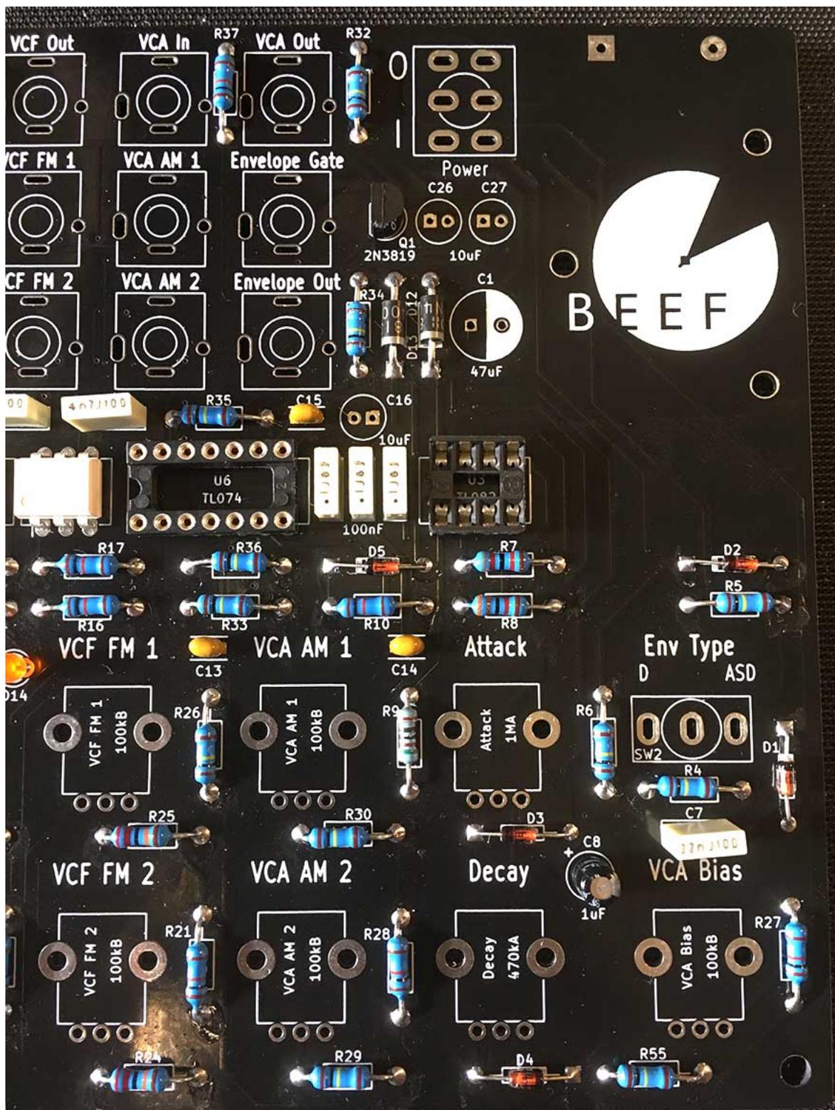
28 - Now place and solder the UNIPOLAR 1uF capacitor at C8. Note: orientation is vital for UNIPOLAR caps! The longer leg must go on the side of the + on the PCB silkscreen.
