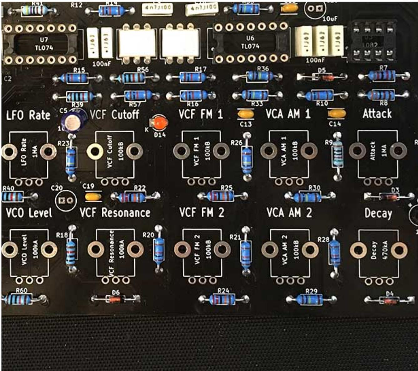
26 - Place and solder the single 2.2uF BIPOLAR cap at C5, located to the right of the LFO Rate text
