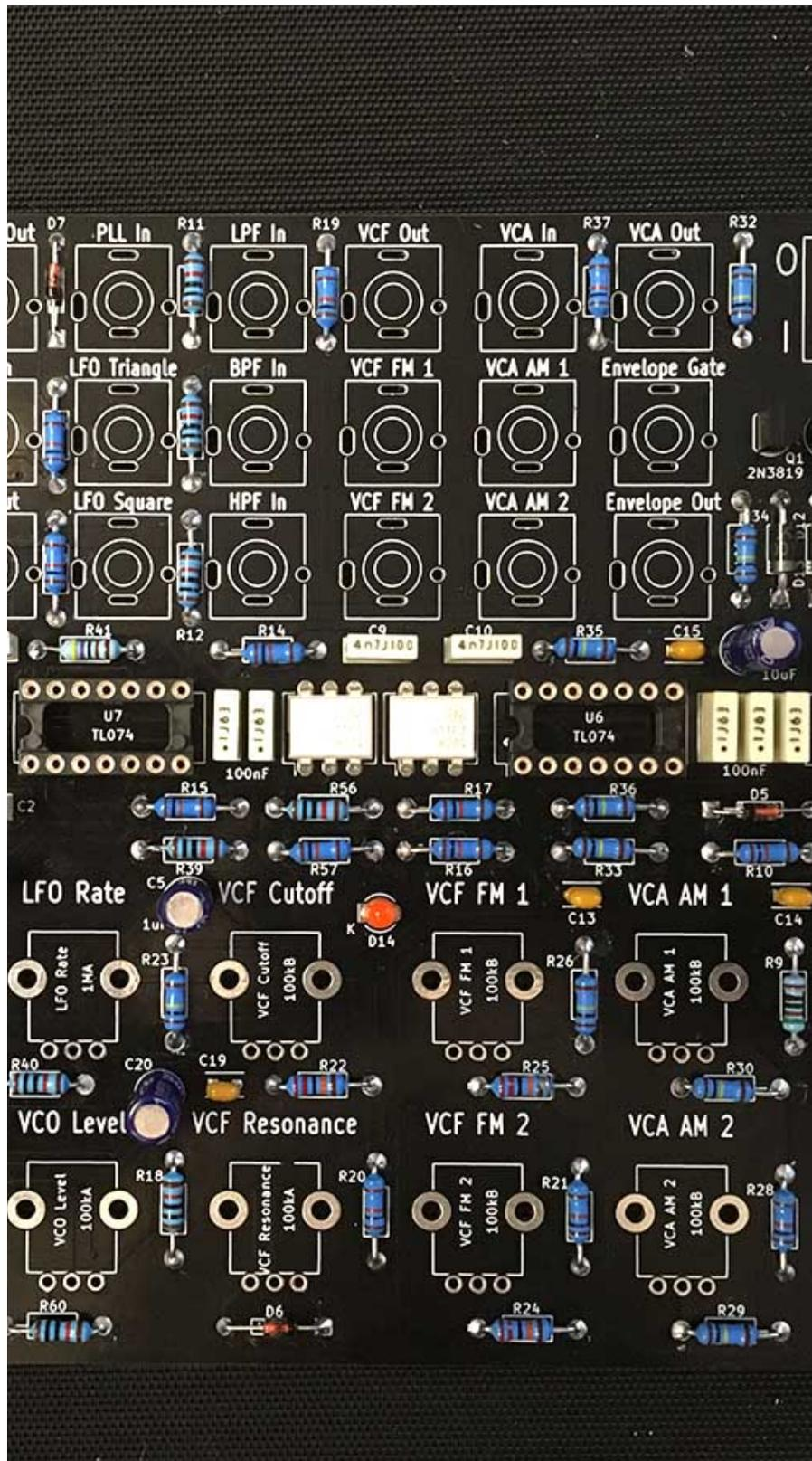
27 - Now place and solder the 2 x 10uF BIPOLAR caps at C16 and C20
