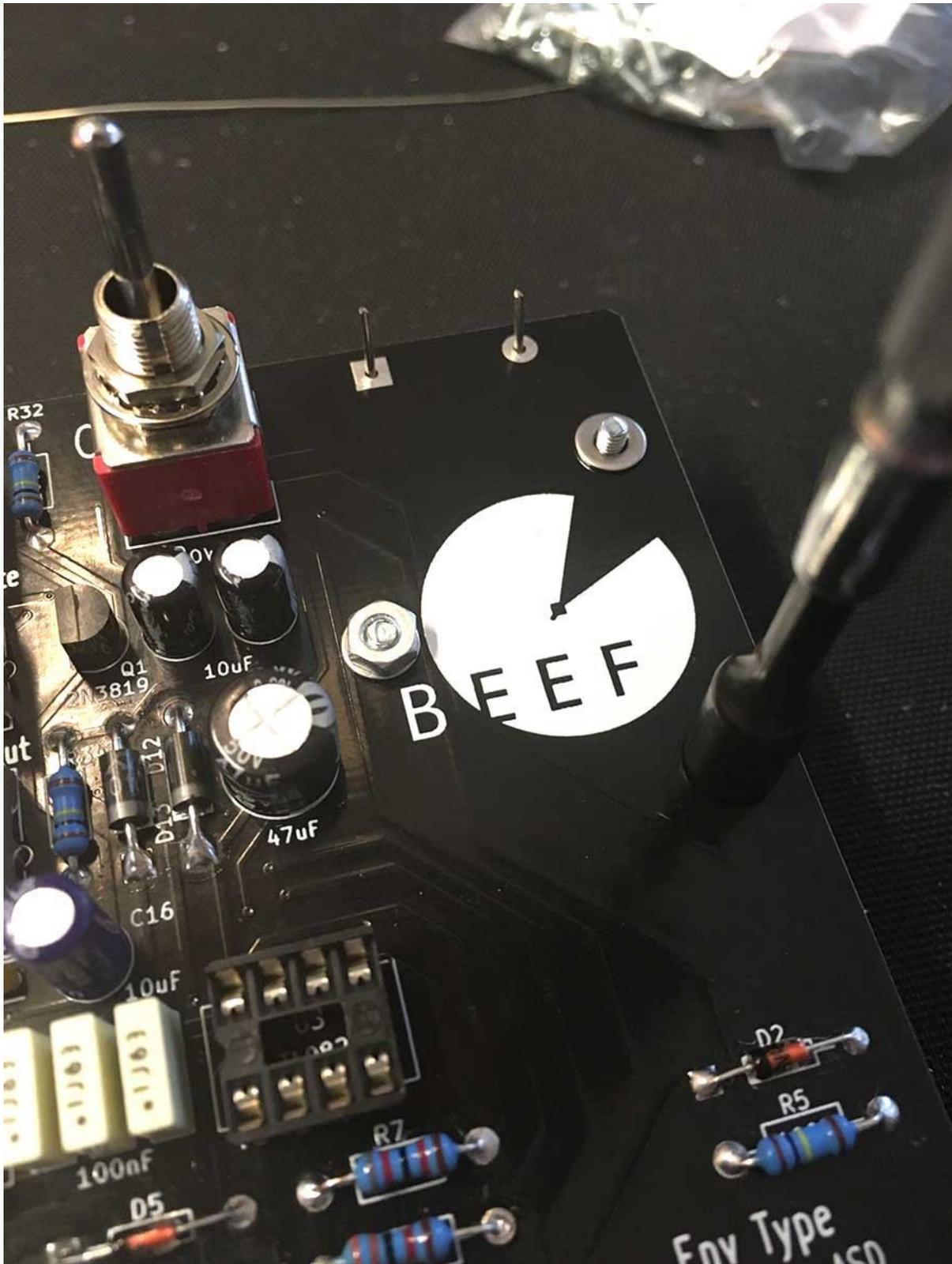
45 – Now you can fit the M2.5 nuts to each screw - a nut driver can make this easier
