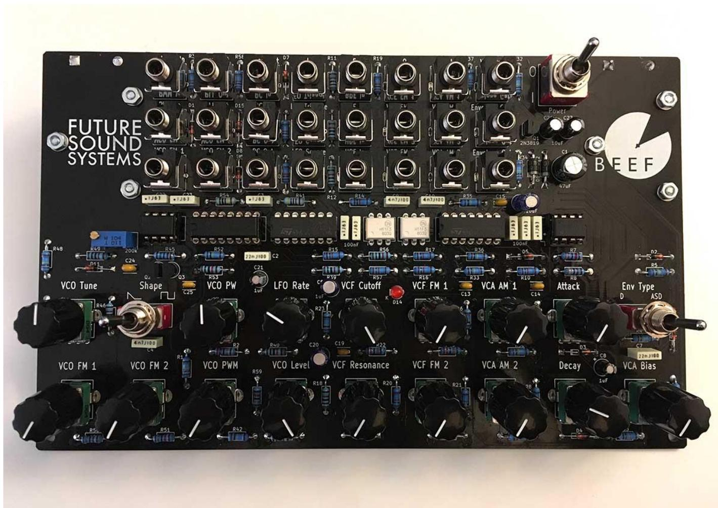
49 - Once you have tested that your build works, you can solder all the remaining legs on the jacks and pots, and then fit the knob caps
