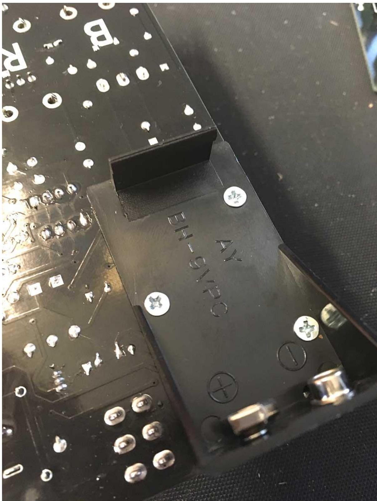
43 - Now fit the two remaining screws into each battery holder
