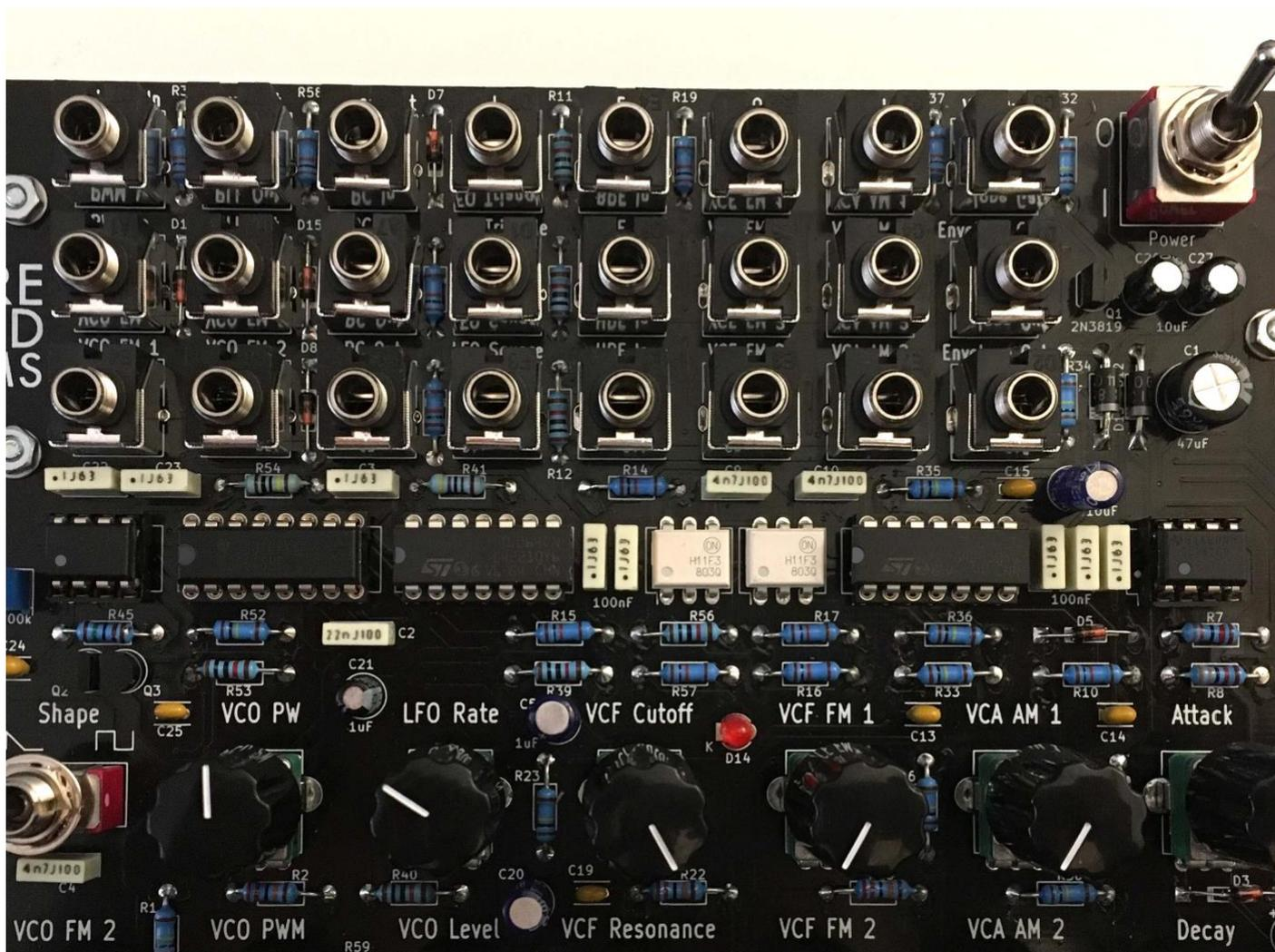
48 - Now paying attention to orientation, fit the IC's to their sockets as shown and fit batteries
